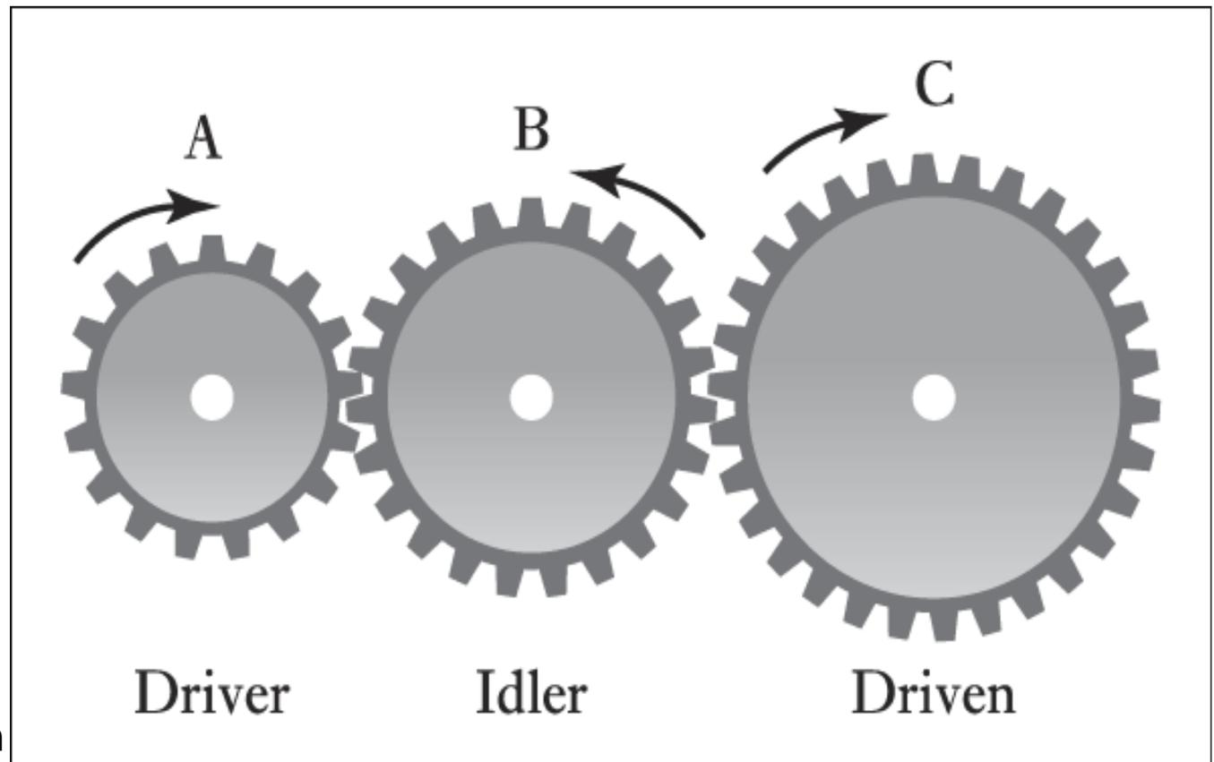
Figure 8.15 Simple gear train
