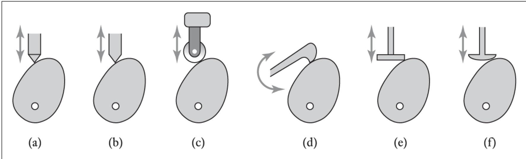
Figure 8.12 Cam followers: (a) point, (b) knife, (c) roller, (d) sliding and oscillating, (e) flat, (f) mushroom
