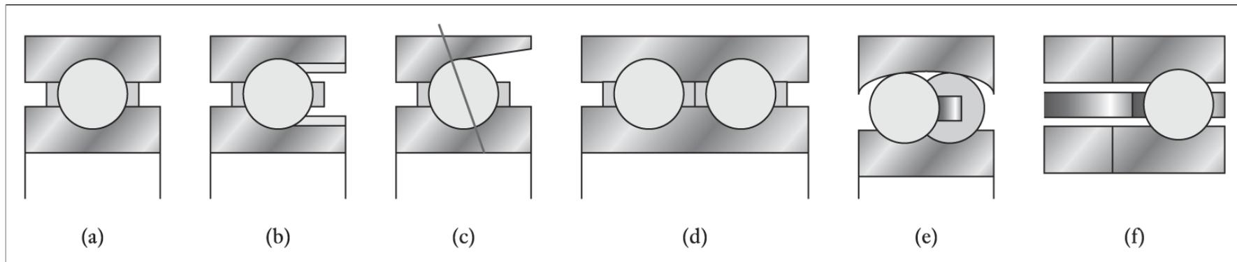
Figure 8.26 Types of ball bearings
