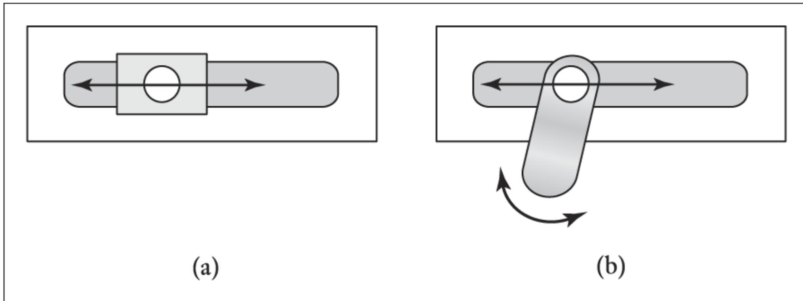
Figure 8.2 Joints with: (a) one degree, (b) two degrees of freedom
