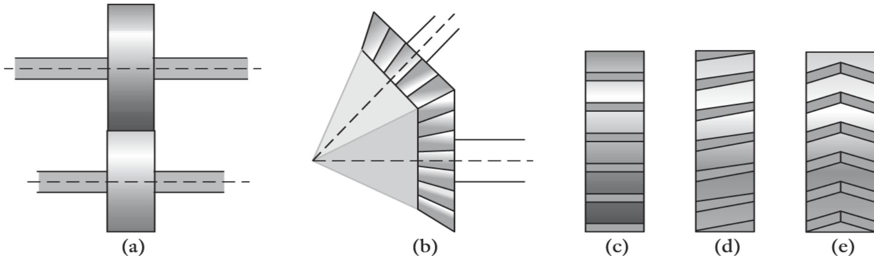
Figure 8.13 (a) Parallel gear axes, (b) axes inclined to one another, (c) axial teeth, (d) helical teeth, (e) double helical teeth
