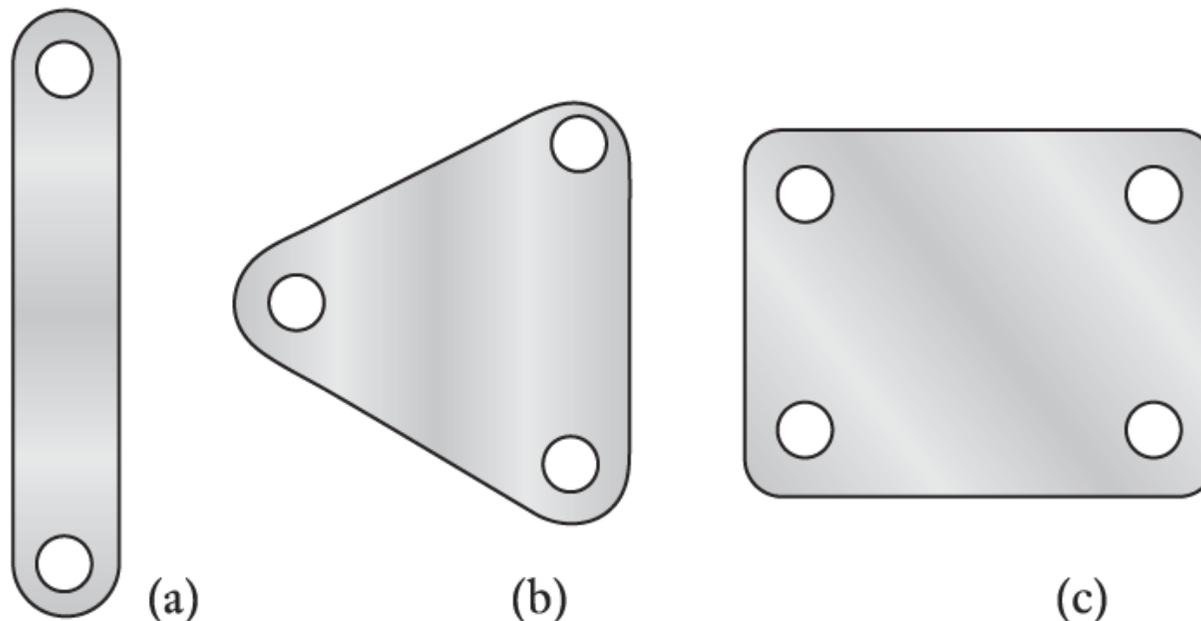
Figure 8.4 Links: (a) with two nodes, (b) with three nodes, (c) with four nodes
