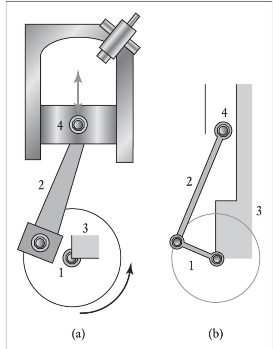
Figure 8.5 Simple engine mechanism
