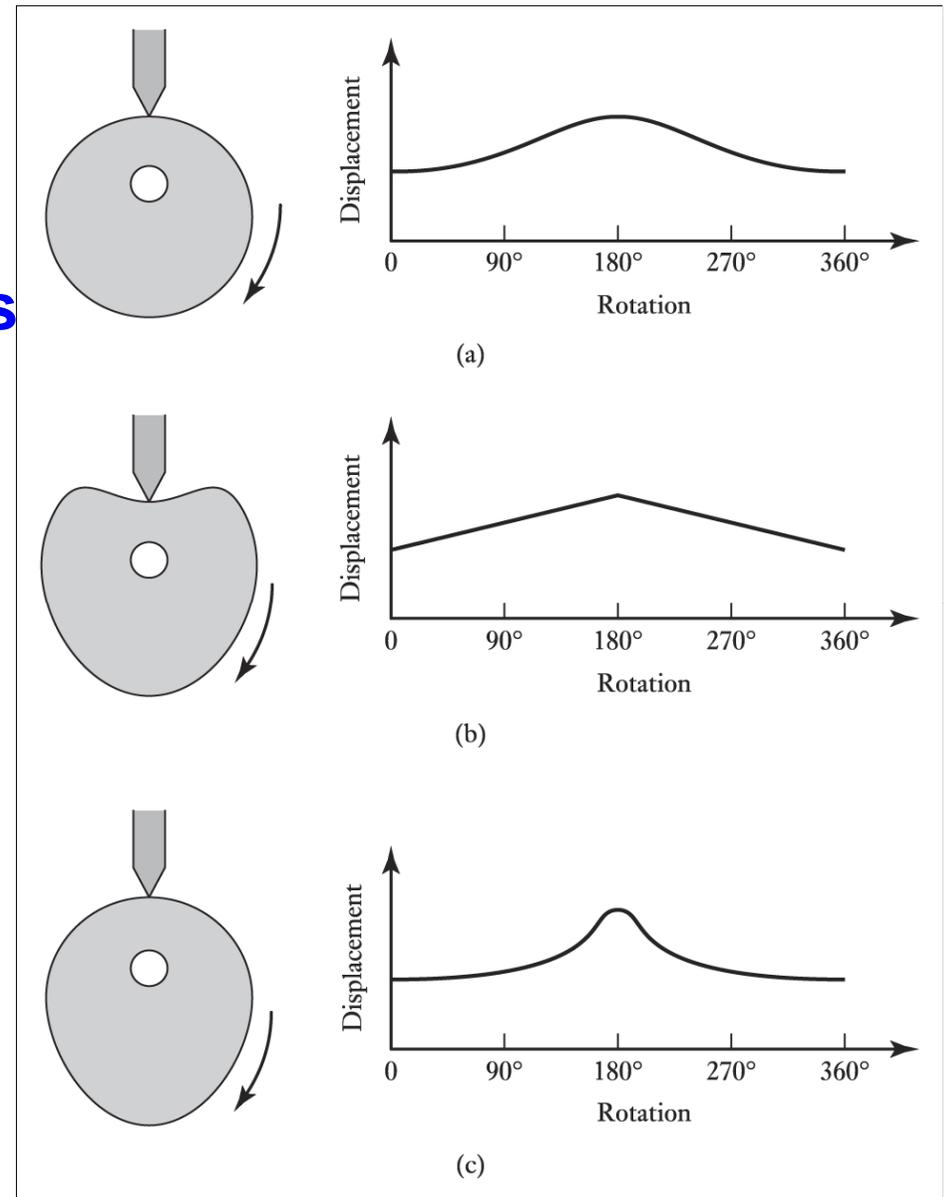
Figure 8.11 Cams: (a) eccentric, (b) heart-shaped, (c) pear-shaped
