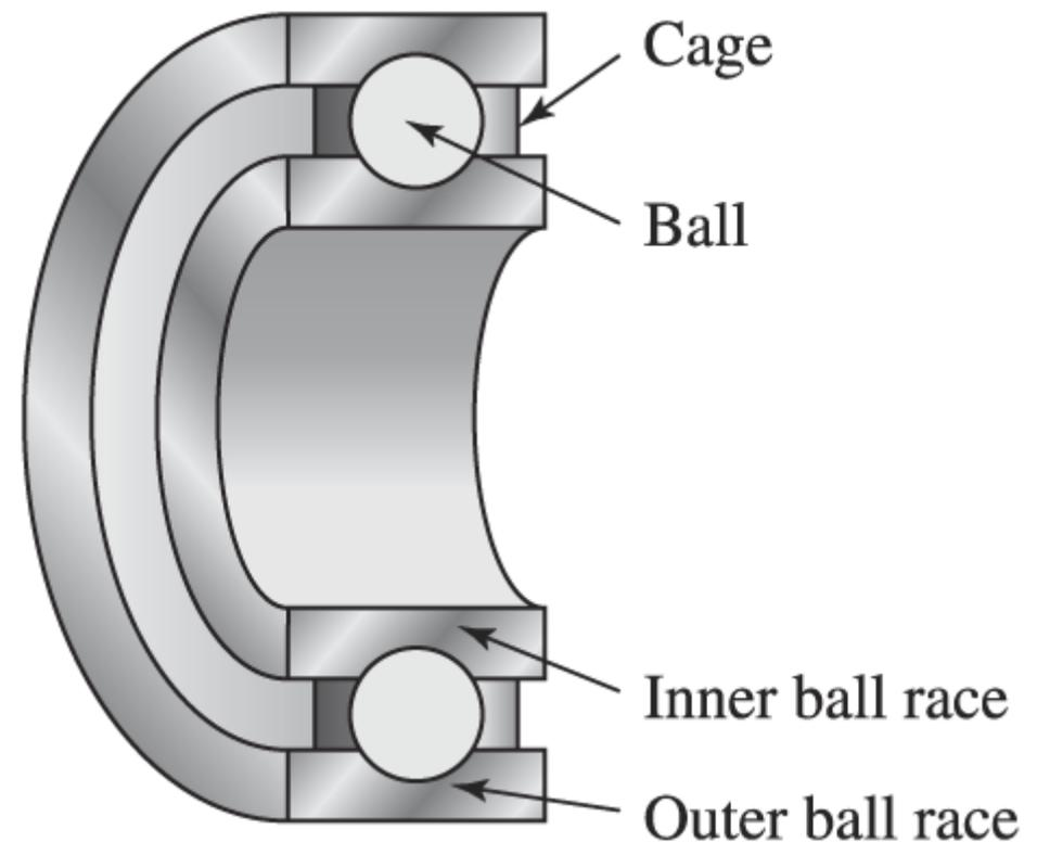
Figure 8.25 Basic elements of a ball bearing
