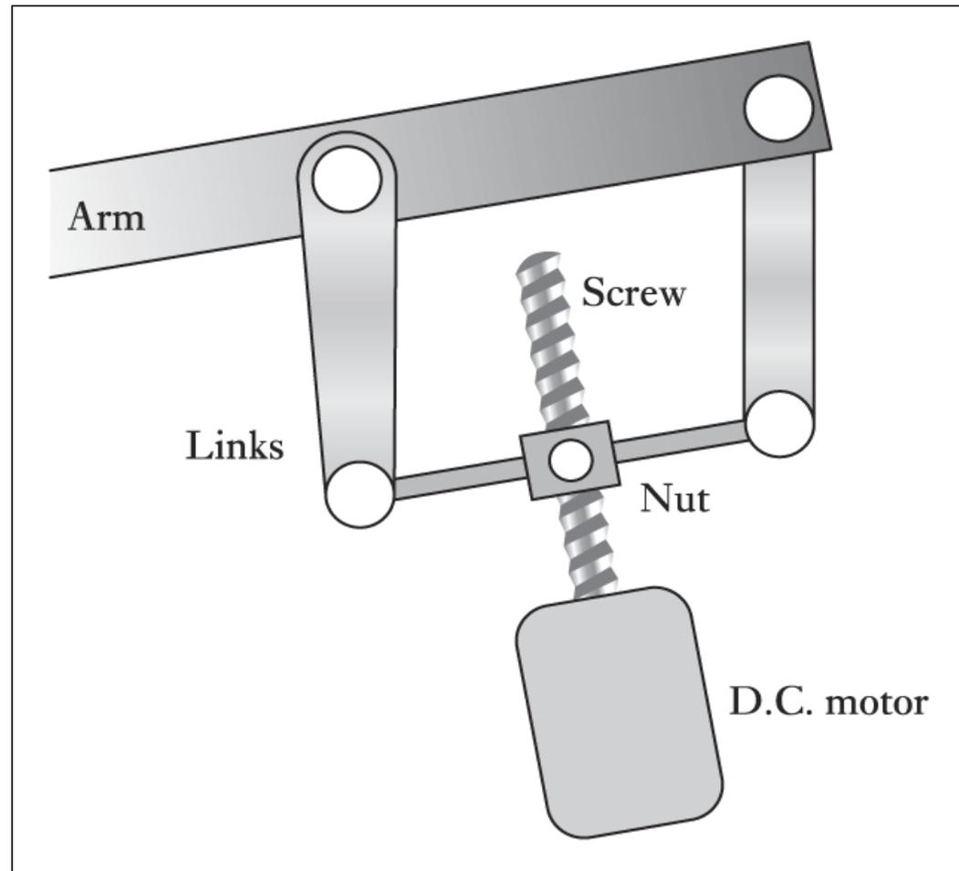
Figure 8.18 Ball screw and links used to move a robot arm
