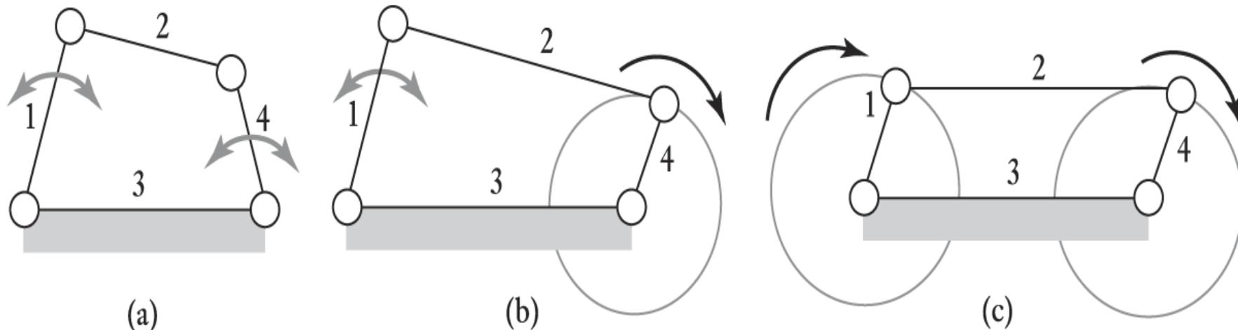
Double lever mechanism **lever crank mechanism**
