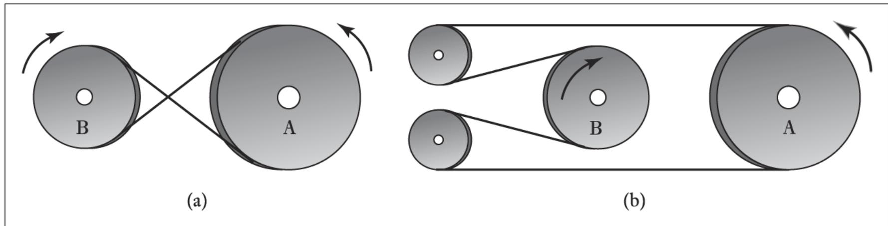
Figure 8.21 Reversed belt drives: (a) crossed belt, (b) open belt
