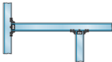
fixed-connected overhanging beam
