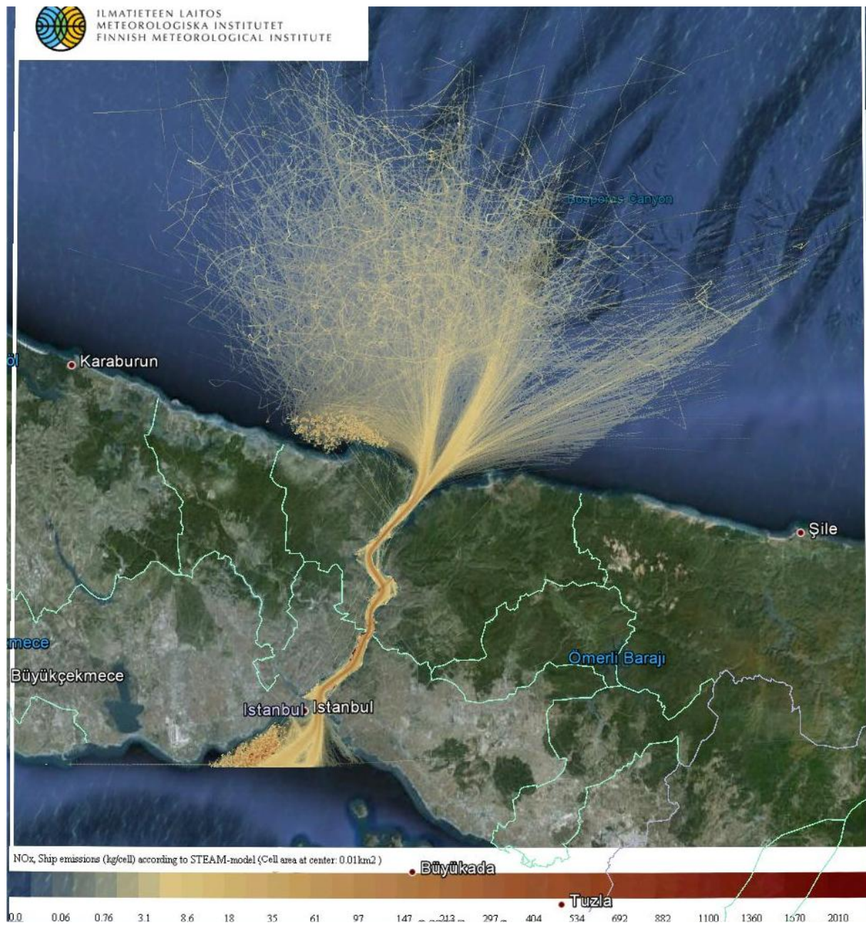
Fig 2: Ship NO x emissions in the Bosphorus area during March 2012 based on AIS data and STEAM model. The scale indicates the total ship emissions in kilograms inside 100 by 100 meter cells.
