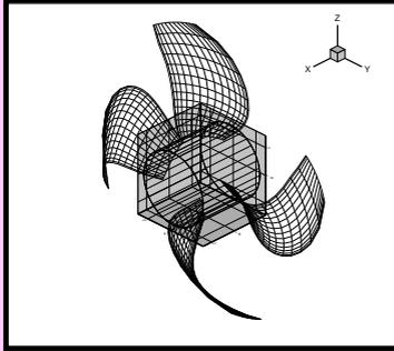
Lifting Surface Design – Wake adapted propeller
