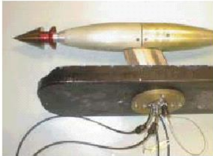
Figure 28: Photograph of model for testing cavitators
