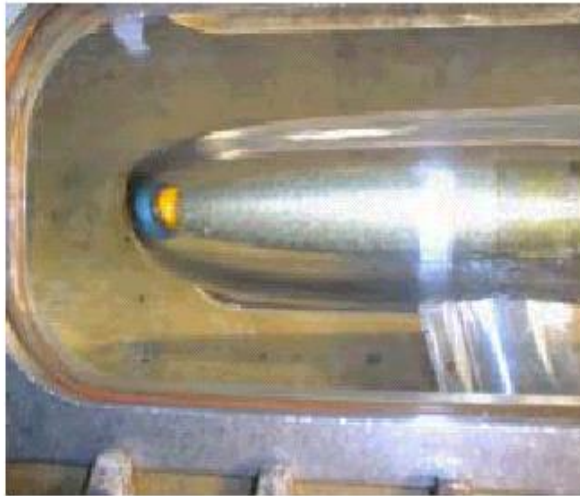
Figure 32: Photograph of cavity formed by a disk at angle of attack
