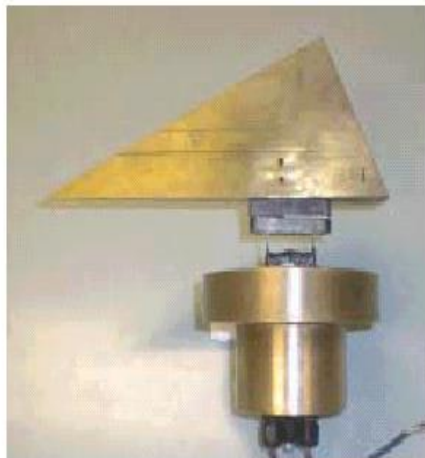
Figure 34: Cavity piercing hydrofoil showing force balance and tunnel mounting fixture
