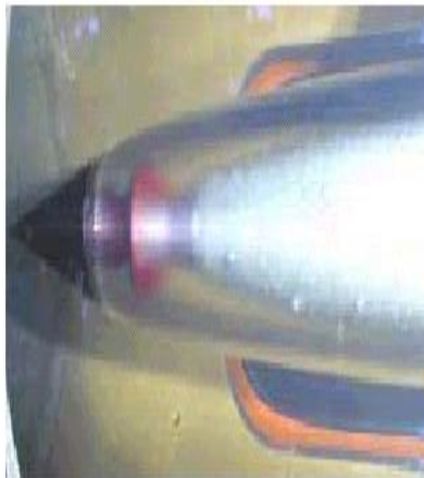
Figure 30: Photograph of cavity formed by a conical nosed cavitator- continuous lighting
