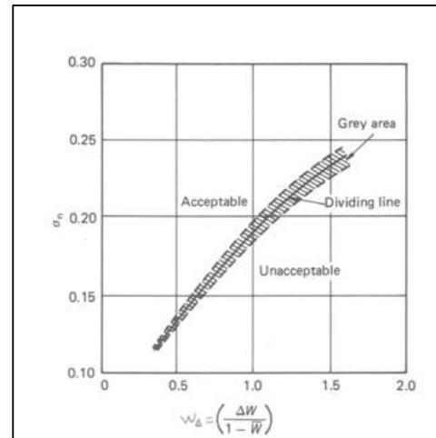
The wake is given in terms of the velocity ratio's method.
