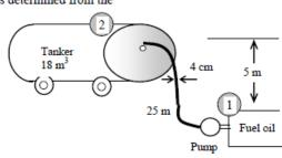
which is greater than 4000. Therefore, the flow is turbulent. The friction factor can be determined from the Moody chart, but to avoid the reading error, we determine it from the Colebrook equation,
