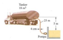
*Analysis* We choose point 1 at the free surface of oil in the reservoir and point 2 at the exit of the hose in the tanker. We note the fluid at both points is open to the atmosphere (and thus  $P_1 = P_2 = P_{atm}$ ) and the fluid velocity at point 1 is zero ( $V_1 = 0$ ). We take the free surface of the reservoir as the reference level ( $z_1 = 0$ ). Then the energy equation for a control volume between these two points simplifies to
