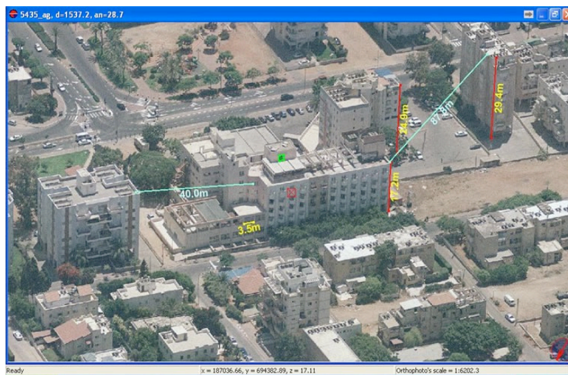
Figure 5. Height and distance measurements (Aeromap, 2006)
