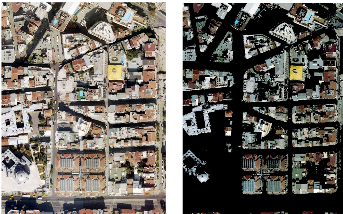
Figure 2: (a) Input multispectral image and automated extracted (b) 2D building objects.
