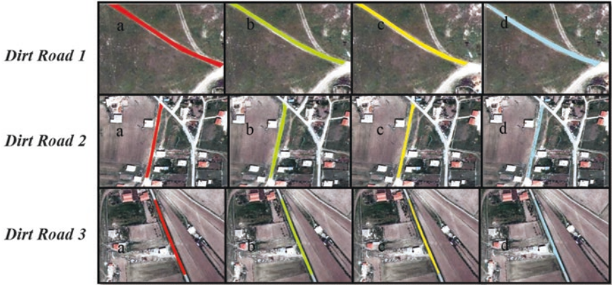
Fig. 7.9 Comparison of dirt roads results: (a) Cadastral data, (b) Manual digitizing, (c) Object based classification and (d) Pixel based classification
