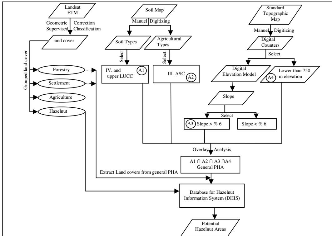
Fig. 6: Flowchart of PHA determination procedure.
