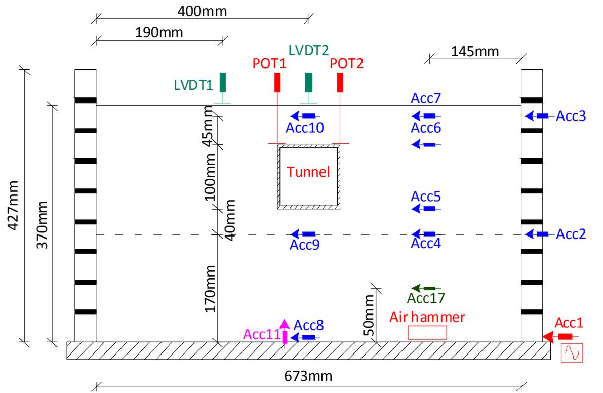
Accelerometer - sensing direction towards left
