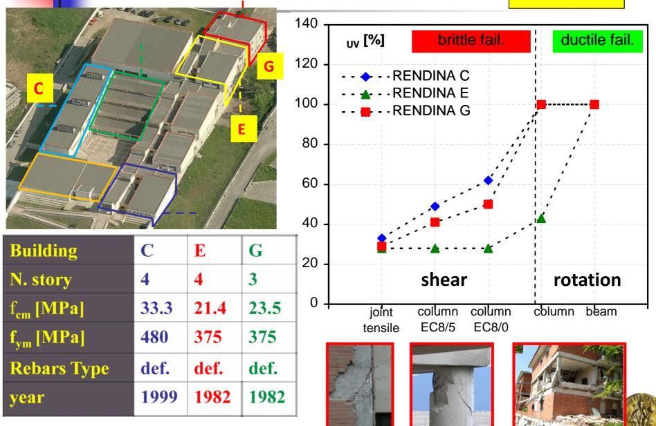
How much FRP based local stengthening interventions could increase the global seismic capacity of existing RC structures?
