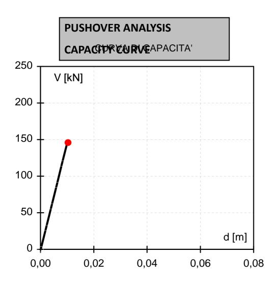
First brittle failure on joint (tensile stress)
