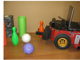
Figure 2: Our Pioneer 3-DX robot grasping one of the objects used in the experiments.
