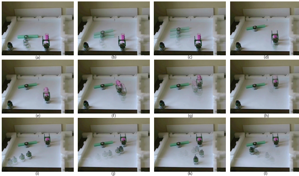
Fig. 3. Khepera II robots achieve the overall mission of pushing/carrying the objects to the final locations and inspecting the area.
