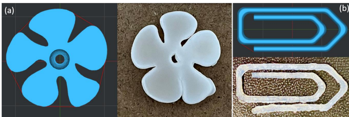
Figure S2. CAD models and real image of the printed flower (a) and paper clip (b) using the hydrogel resin.
