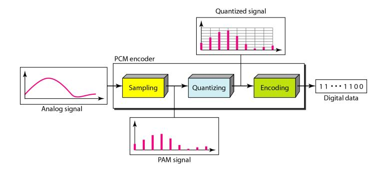
• The sampling results in a discrete set of digital numbers that represent measurements of the signal
