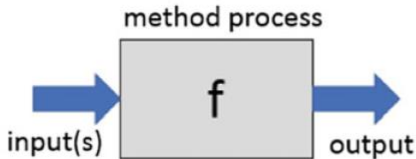
A black box model with input(s) and an output
