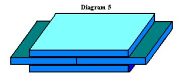
The rivets to be used have a diameter of 3/4 inch. The maximum allowable stresses for the rivet and plate materials are as follows:
