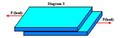
Rivets:  $T = 20,000 \text{ lb/in}^2$ ,  $\sigma_t = 21,000 \text{ lb/in}^2$ ,  $\sigma_c = 23,000 \text{ lb/in}^2$
