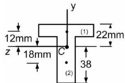
$$I_{zz} = I = 868 \times 10^3 \text{ mm}^4 = 868 \times 10^{-9} \text{ m}^4$$
