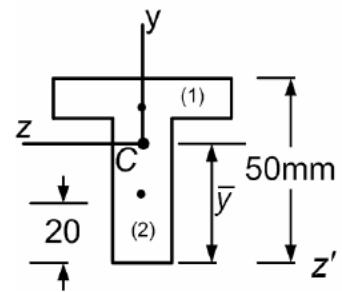
$$A\bar{y} = \sum \bar{y}A \Rightarrow \bar{y}3000 = 114 \times 10^3 \Rightarrow \bar{y} = 38 \text{ mm}$$
