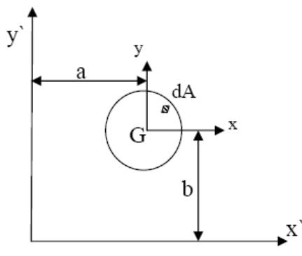
$$\left. \begin{array}{l} I_{x'} = \int y'^2 dA \\ I_{y'} = \int x'^2 dA \\ I_{xy'} = \int x'y' dA \end{array} \right\} \text{bilinmiyor} \quad \left. \begin{array}{l} I_x = \int y^2 dA \\ I_y = \int x^2 dA \\ I_{xy} = \int xy dA \end{array} \right\}$$
