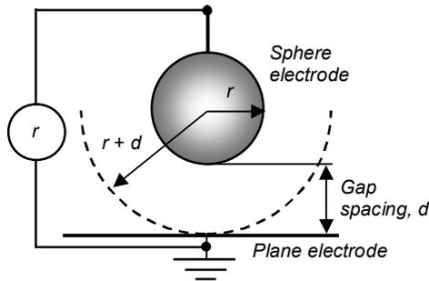
**Figure 1:** The sphere-plane electrode system.
