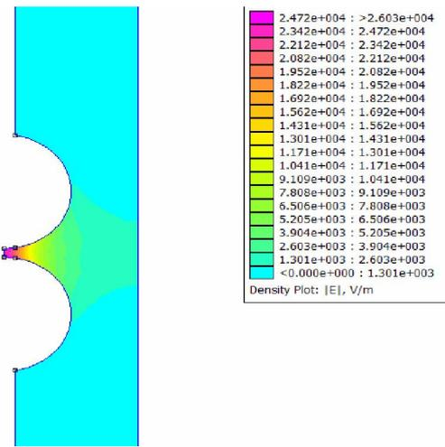
**Figure 2:** The electric field distribution in sphere-sphere electrode configuration.
