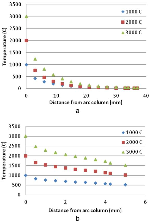
**Figure 7:** Electrode temperature dissipation with respect to distance from arc column: a) plane electrode; b) rod electrode
