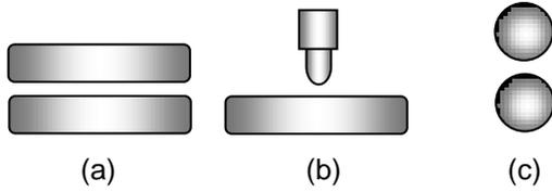
**Figure 1:** Used electrode types: a) plane-plane; b) rod-plane; c) sphere-sphere electrodes
