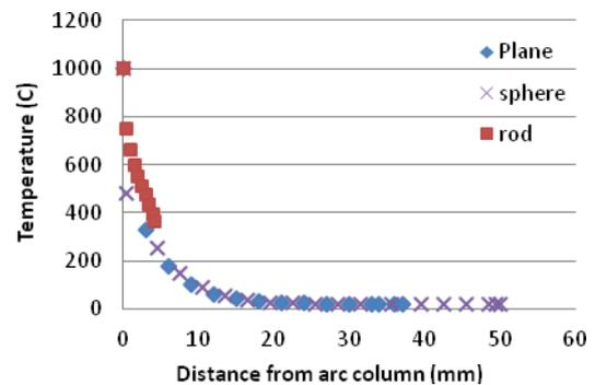
**Figure 6:** Surface temperature distribution for the different electrodes
