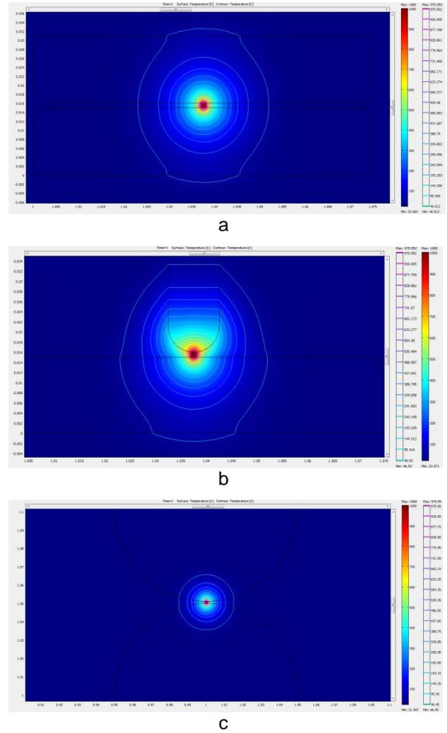
**Figure 2:** Temperature distributions of electrode systems: a) plane-plane; b) rod-plane; c) sphere-sphere electrodes
