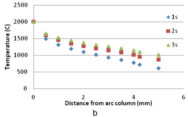
**Figure 8:** Electrode temperature dissipation with respect to distance from arc column: a) plane electrode; b) rod electrode
