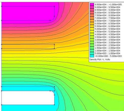
Fig. 6. Potential distribution (one of the barriers located between the electrodes)
