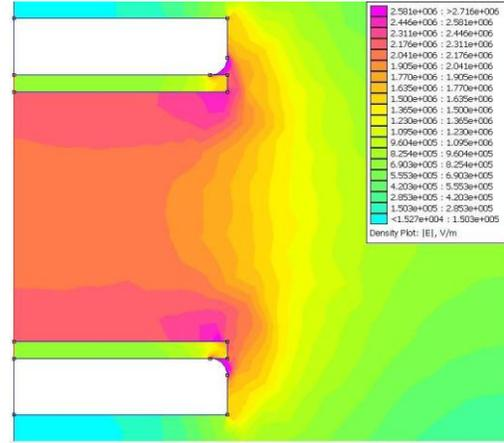
Fig. 7. Electric field distribution for case of insulating barriers on the electrodes
