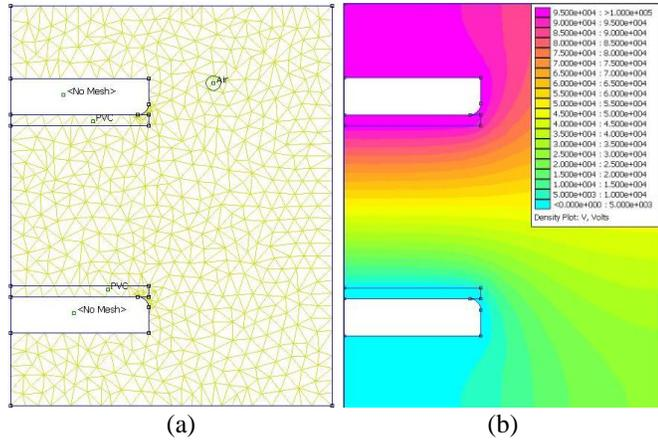
Fig. 5. (a) Geometry and finite element mesh, and (b) Potential distribution of the problem (insulating barriers on the electrodes)
