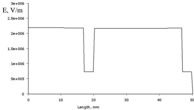
Fig. 9. Variation of electric field intensity along gap length for case of one of two barriers located on the electrode.
