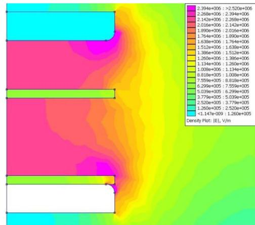
Fig. 8. Electric field distribution for case of one of the barriers located between the electrodes
