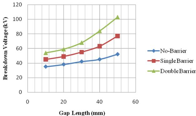
Fig. 3. Breakdown voltage of air under positive DC voltage
