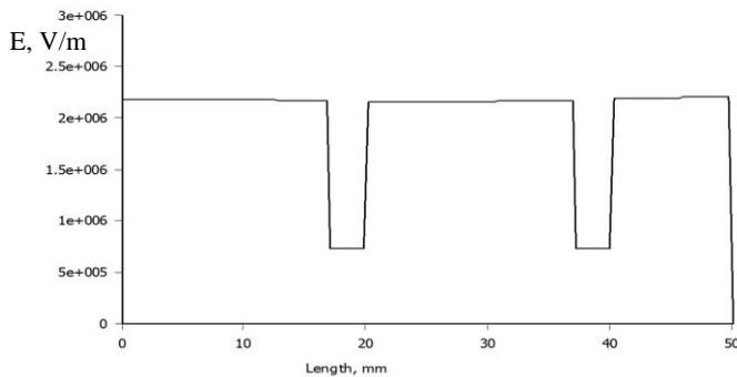
Fig. 10. Variation of electric field intensity along gap length for case of the barriers located between the electrodes
