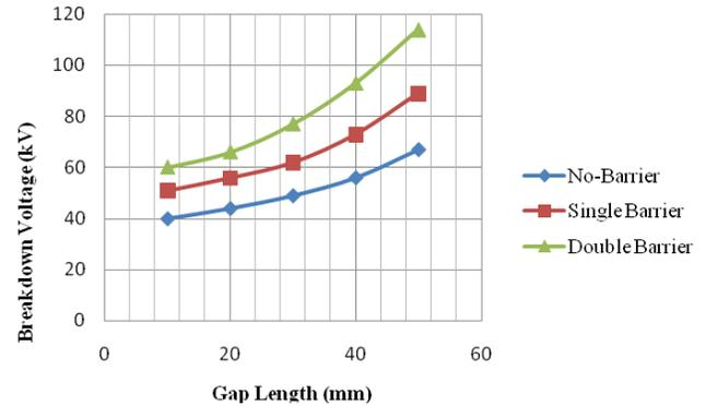
Fig. 4. Breakdown voltage of air under negative DC voltage
