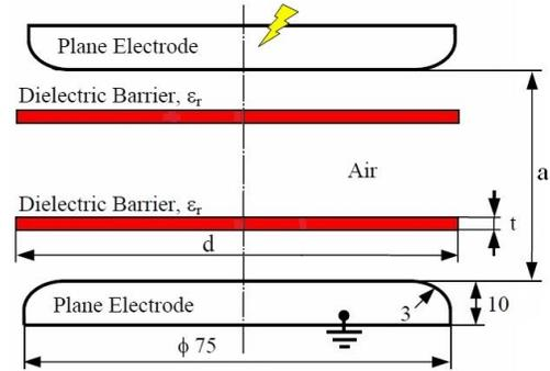
Fig. 1. Electrode configuration (dimensions in mm)
