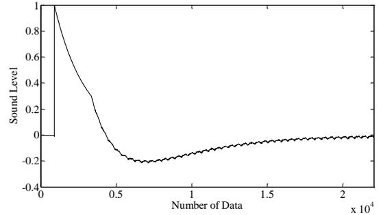
Fig. 2. The first 22050 data of the positive DC corona sound for 1 second at 50 kV.
