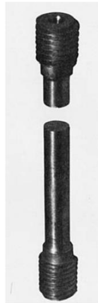
Photo 2.5 Tested specimen of a brittle material.
