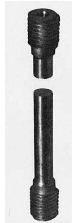
Photo 2.5 Tested specimen of a brittle material.
