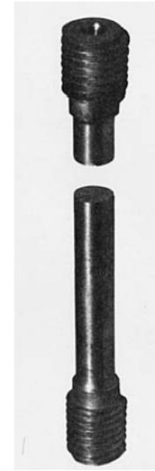
Photo 2.5 Tested specimen of a brittle material.
