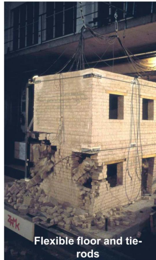
Brick masonry building models after shaking table tests
