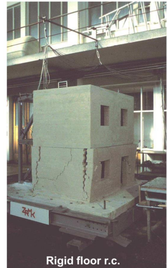
Brick masonry building models after shaking table tests
