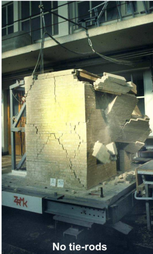
Brick masonry building models after shaking table tests
