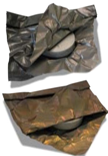
Workpieces in foil heat treating
