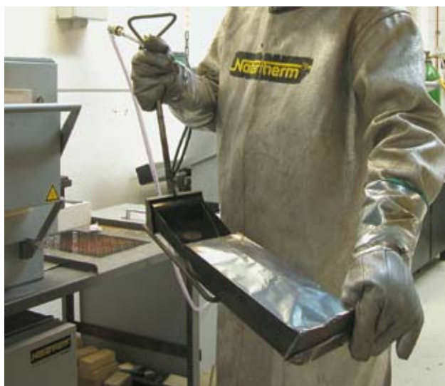
Protective gas annealing bag in operation
