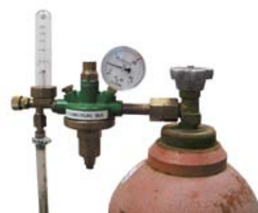
Pressure reducing valve with assembled flow meter
