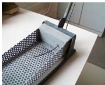
Thermocouple integrated in holder
