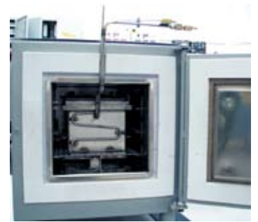
Air circulation furnace with protective gas box
