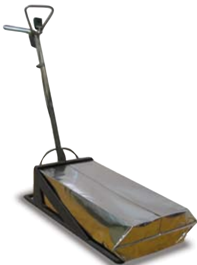
Holder with protective gas annealing bag
