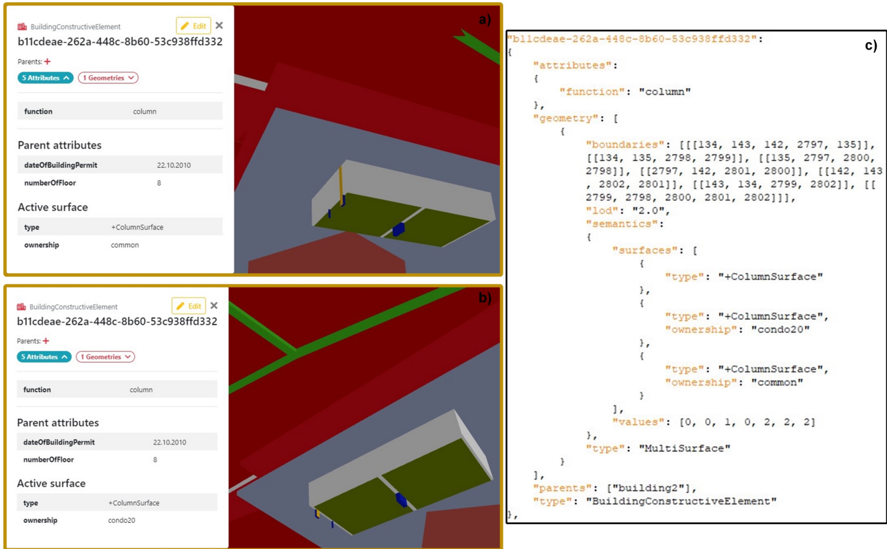
Figure 11. The semantic surface examples on a column and their details: a) +ColumnSurface representing common ownership, b) +ColumnSurface representing private ownership, c) corresponding part of the CityJSON file for the column object.
