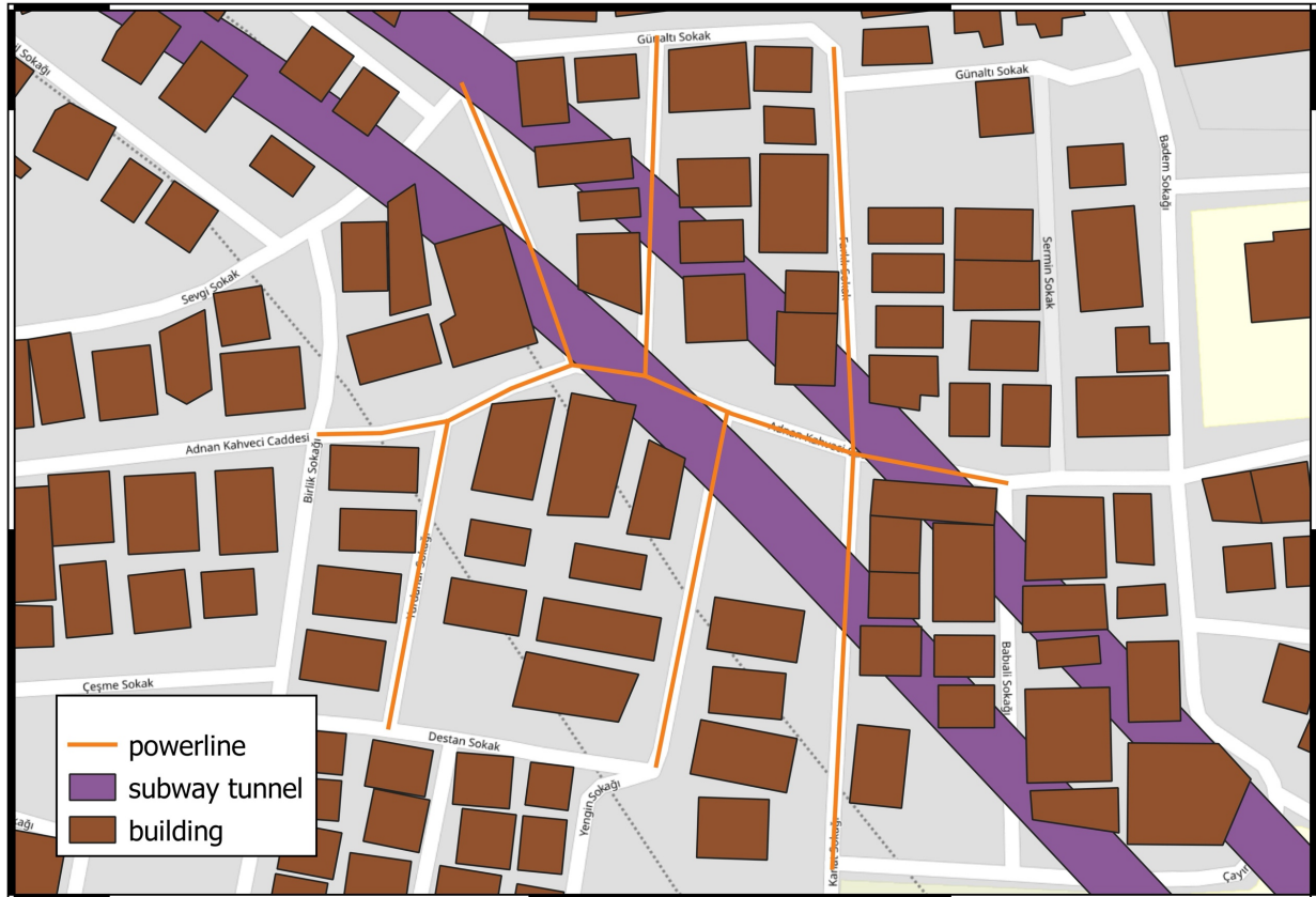
Figure 5. 2D map representing the situation regarding the powerline network and subway tunnels.
