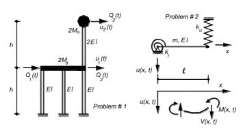
of the beam is fixed and has a rotational spring  $k_t$ . The right end of the beam is free and has a lateral spring  $k_u$ . Write down the boundary conditions for the free vibration of the beam. Obtain the frequency determinant in terms of  $\beta^4 = m\ell^4\omega^2/(EI)$   $\beta = m\ell^4\omega^2/(EI)$  by assuming  $M_o = m\ell$ ,  $k_u = EI/\ell^3$  and  $k_t = EI/\ell$ .
