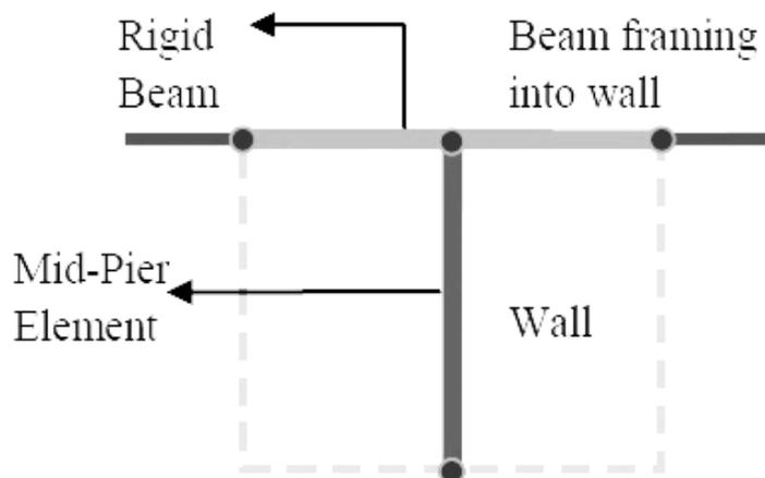
**Figure 5.** Mid-Pier model for shear wall
