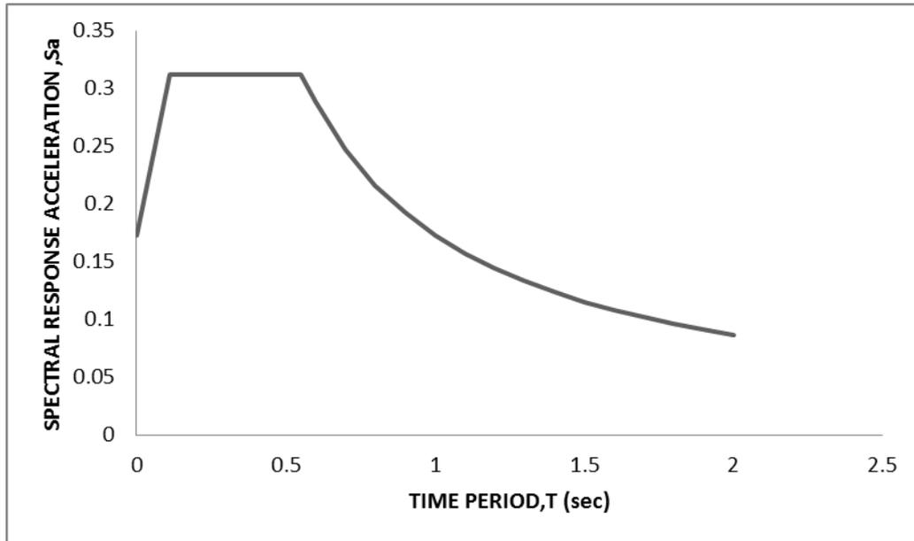
**Figure 2.** Design response spectrum used in the analysis (SBC 301,2007)
