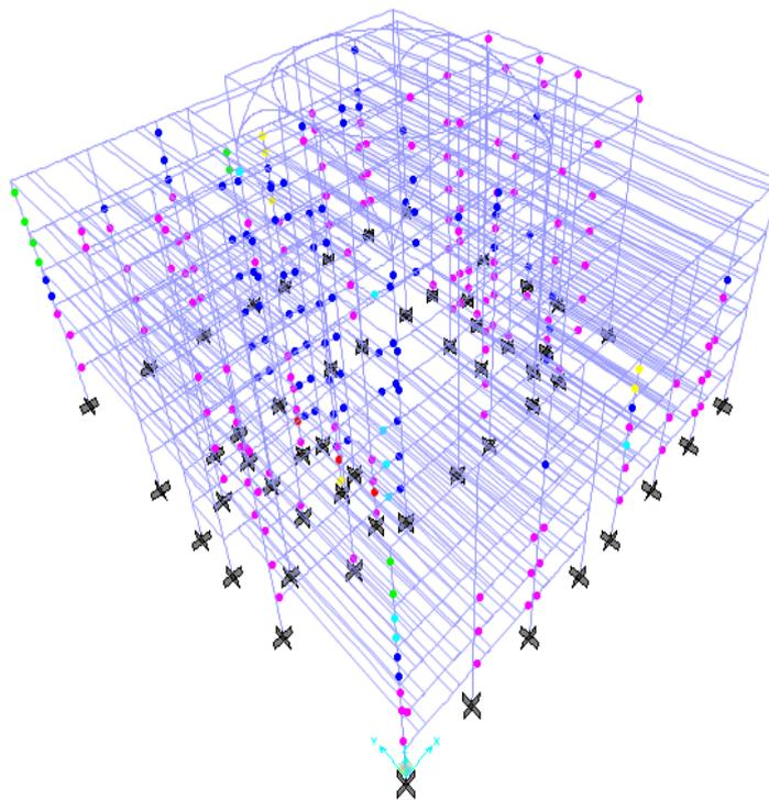
**Figure 9.** Plastic hinges status when pushed in negative x – direction
