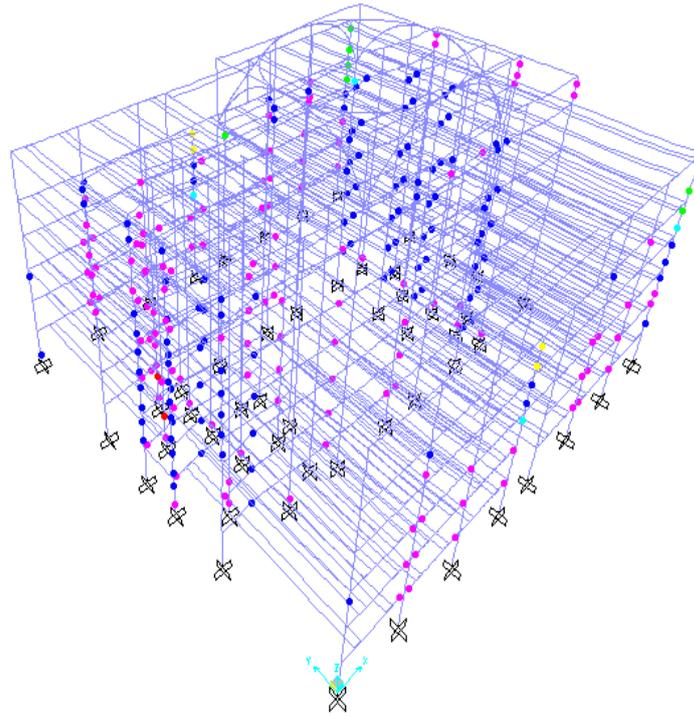
**Figure 8.** Plastic hinges status when pushed in positive x – direction
