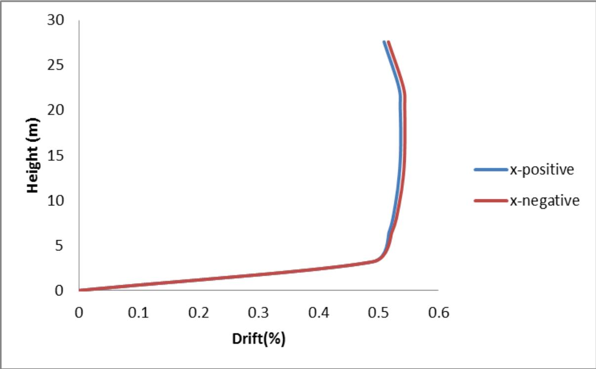
Figure 7. Storey drift ratio of the building
