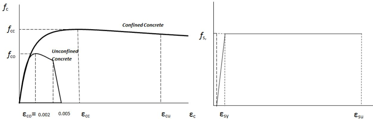
**Figure 4.** Mander Unconfined, Confined Model and Elastoplastic Steel Model
