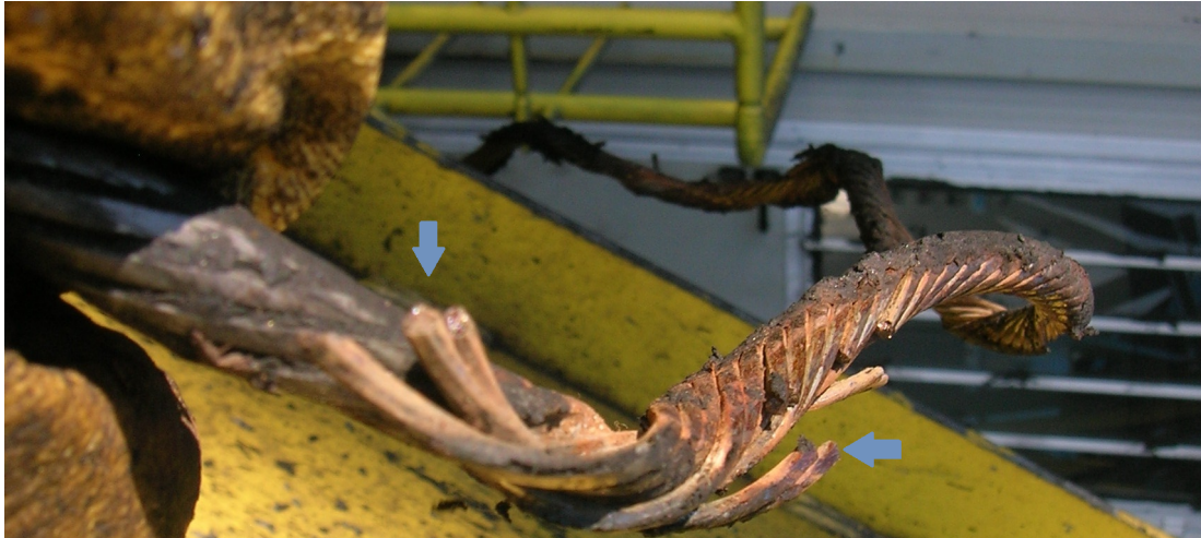
Figure 4.1 : A damaged wire rope.
