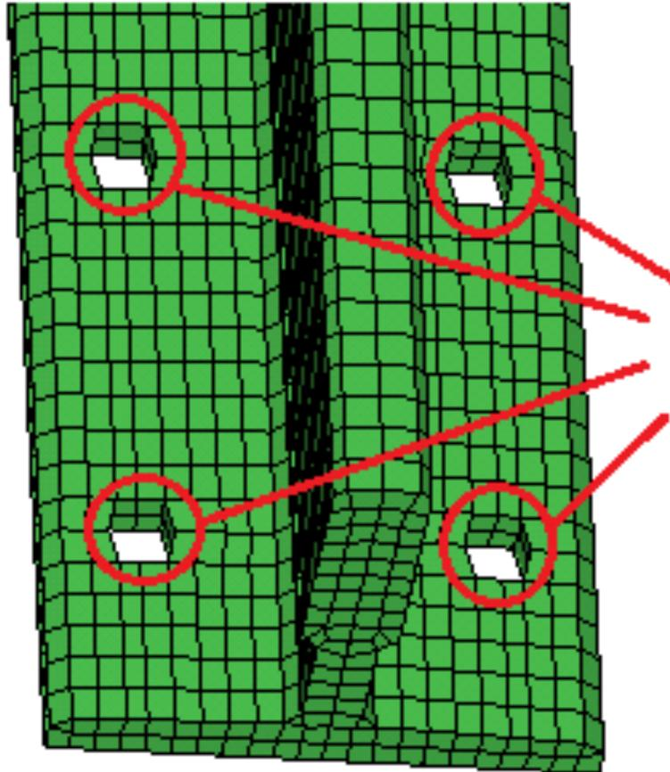
a) Connection nodes between rail and brackets
