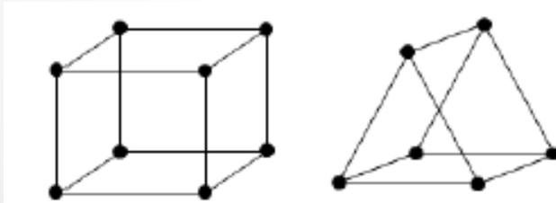
Rectangular prism elements with 8 node points and triangle prism elements with 6 node.
