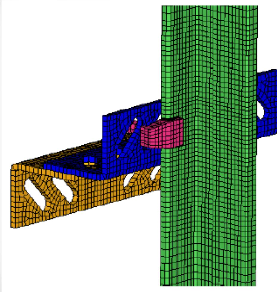
The stress and deformation calculations of guide rail (T90) have been performed according to EN-81-1:1998 standard during safety gear operation.
