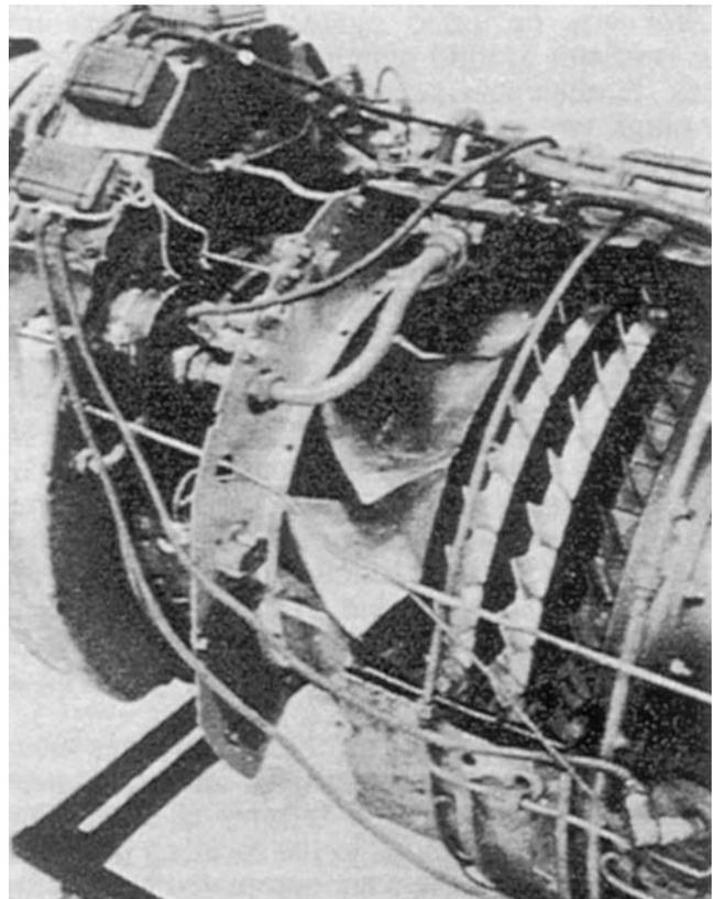
Figure 64. Compressor Section of the HeS 011 Engine Showing the Unique Diagonal Mixed Flow Compressor. (Bentele, 1991)
