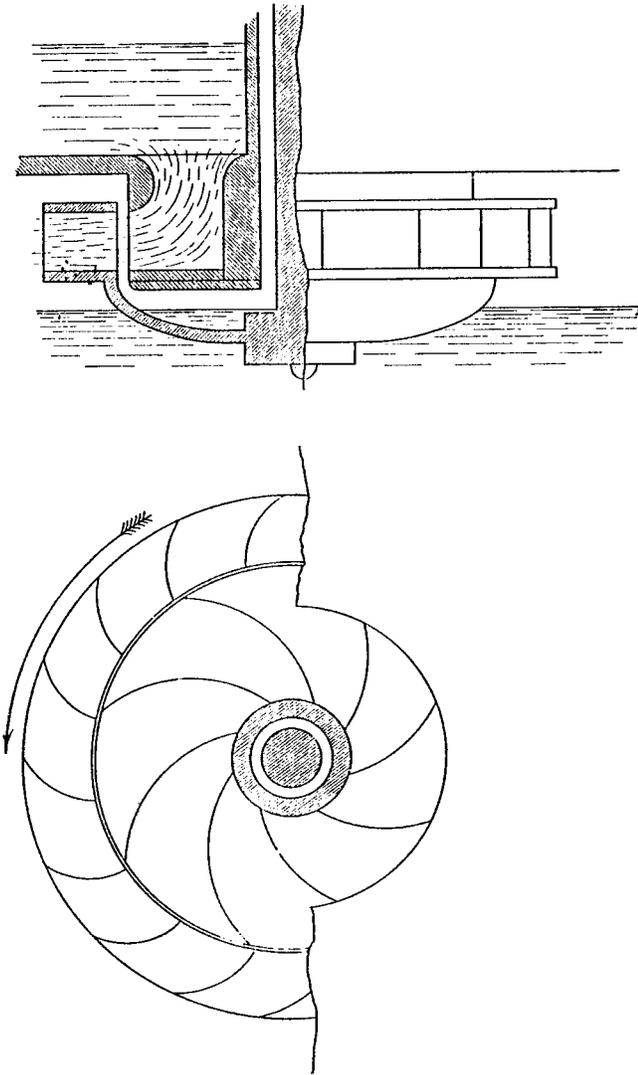
Figure 6. Fourneyron's Hydraulic Turbine-Radial Outflow Design with Inlet Guide Vanes. (Garnett, 1906)
