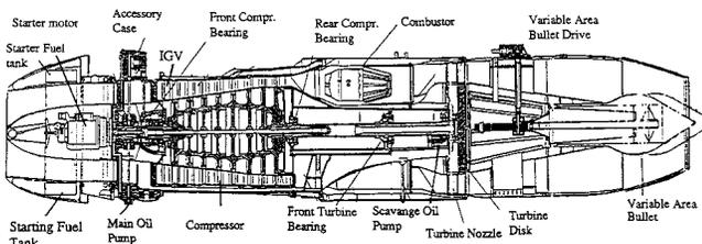
Figure 70. Cross Section of the Junkers Jumo 004 Turbojet Showing Eight-Stage Axial Compressor, Six-Can Annular Combustors, and Single-Stage Air-Cooled Turbine. (Neville and Silsbee, 1948)
