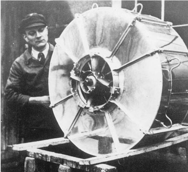
Figure 53. Von Ohain's Prototype Turbojet Built in 1934. (Bentele, 1991)
