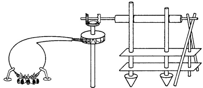
Figure 3. Impulse Turbine of Giovanni Branca Used to Power a Stamping Mill, Circa 1629—Possibly the Earliest Steam Turbine.
