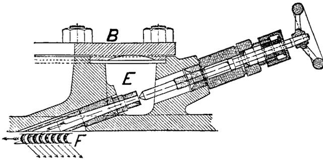
Figure 10. De Laval Steam Turbine Nozzle and Vane. (Kennedy, 1910)
