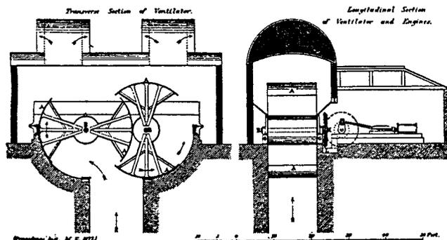
Figure 24. Early Roots Blower Used for Mine Ventilation. (Early Roots Brochure, Undated)
