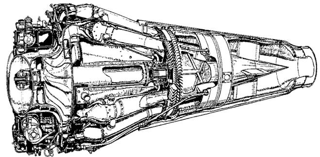
Figure 50. De Havilland Goblin Engine (Rated at 3000 Lb Thrust, 10,200 RPM, Weight 1550 Lb) Used on the Vampire Jet Fighter. Unlike the Whittle Designs, It Used a Single-Sided Centrifugal Compressor. (Geoffrey Smith, 1946)
