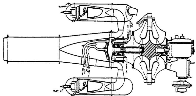
Figure 35. Engine Layout of Third Experimental Unit with 10 Reverse Flow Combustors. (Meher-Homji, 1997; Courtesy ASME)
