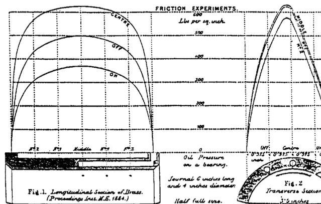
Figure 75. Beauchamp Tower's Experimental Results in Measuring Oil Film Pressure.
