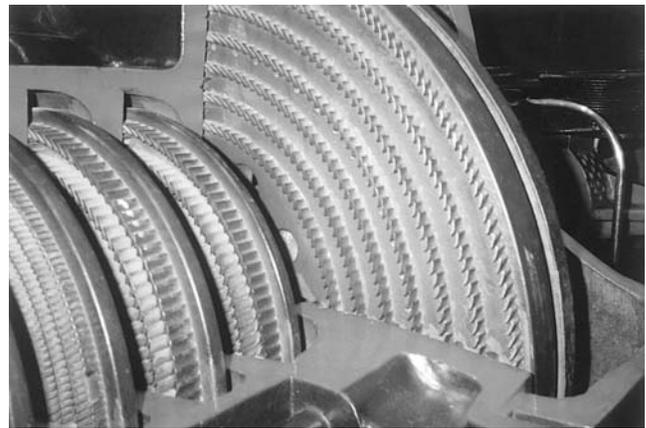
Figure 18. Blade Details of Parsons' Radial Flow Turbine.
