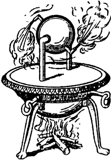
Figure 1. Aeolipile Developed by Hero of Alexandria 120 BC. (Sawyer, 1945)
