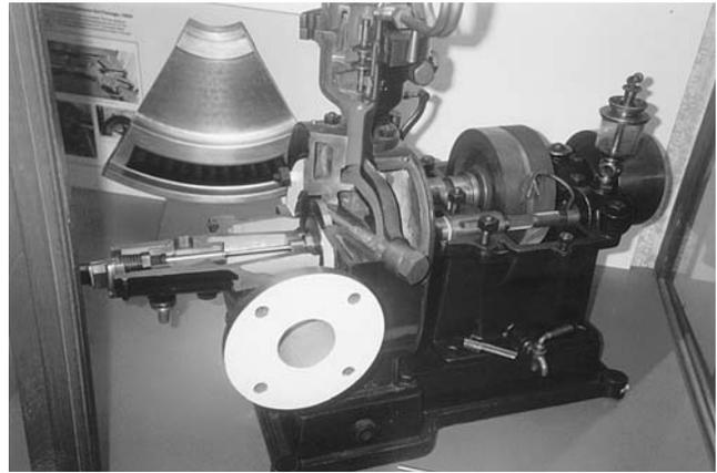
Figure 13. High-Speed De Laval Turbine Sectioned View Including Reduction Gearing.
