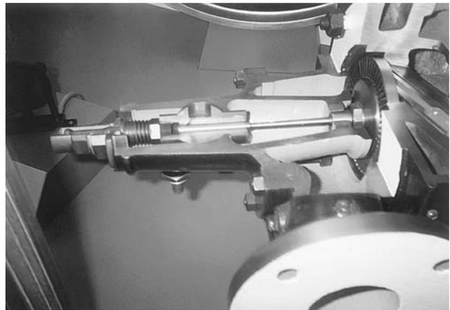
Figure 14. Detail View of De Laval Steam Turbine Showing Flexible Shaft and Bearing Arrangement.
