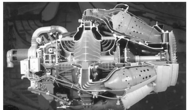
Figure 40. Sectioned Photo of Rolls Royce Nene Engine. (Courtesy Doug Nagy, Liburdi Engineering Limited)
