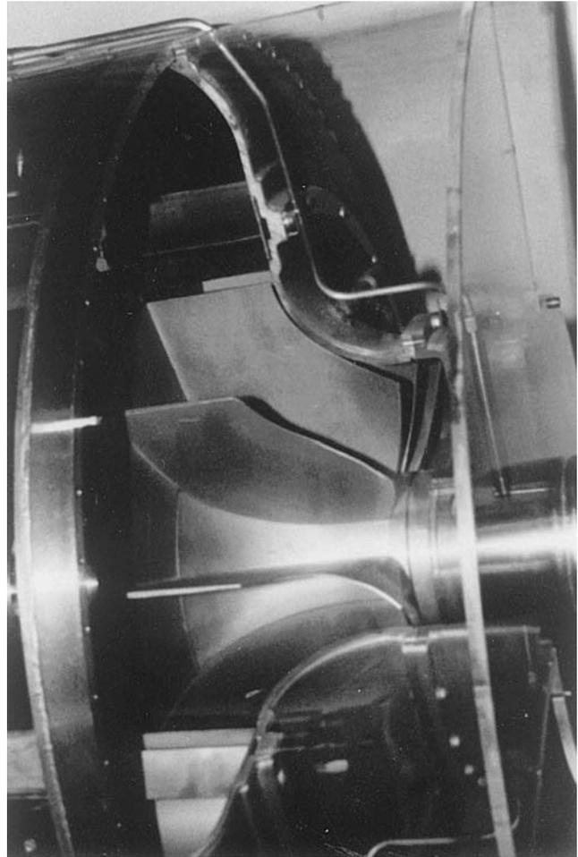
Figure 58. Radial Inflow Turbine of the HeS 3B Engine. (Meher-Homji, 1999; Courtesy ASME)
