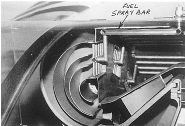
Figure 57. Wraparound Combustor of the HeS 3B Engine Showing Fuel Spray Bar. (Meher-Homji, 1999; Courtesy ASME)
