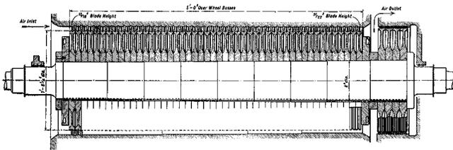
Figure 26. 48-Stage, Axial Flow Compressor Made by Parsons in 1904. (Flow rate 3000 cfm, Discharge pressure 8 to 15 psig, 3600 rpm.) (Parsons, 1926)
