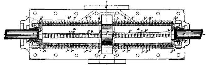
Figure 16. Sectional View of First Parsons Axial Steam Turbine Rated at 10 HP, 18,000 RPM. (Parsons, 1926)
