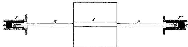
Figure 74. Patent Drawing (May 1889) of De Laval Flexible Shaft and Bearing.
