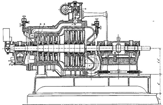
Figure 22. Cross Sectional View of Rateau Steam Turbine. (French, 1908)
