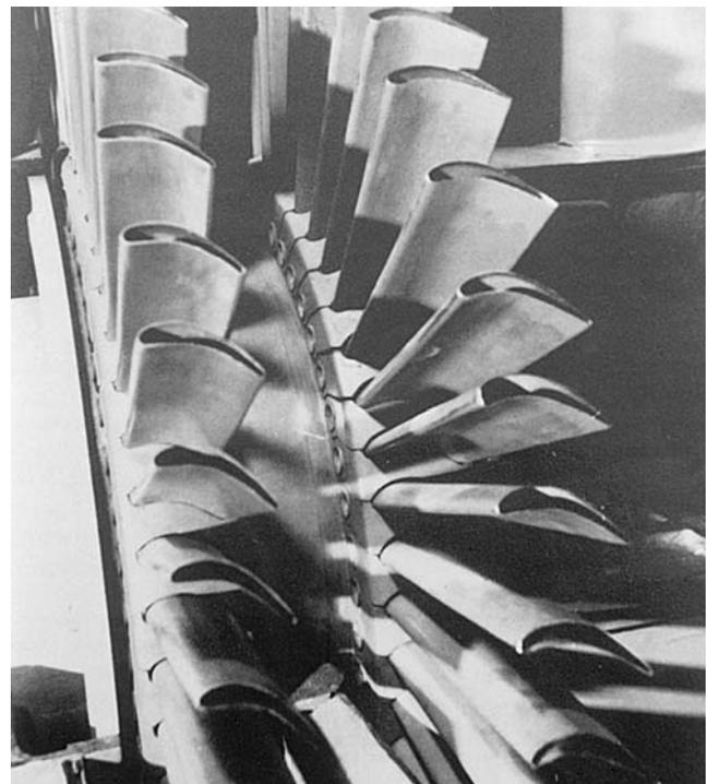
Figure 65. Details of the Advanced Air-Cooled Turbine Section Designed by Dr. Max Bentele for the HeS 011 Engine. (Bentele, 1991)
