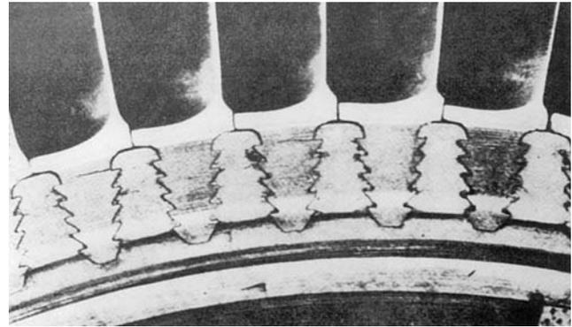
Figure 46. Cracking of Turbine Blade Root Serrations, W.1A Turbojet. (Development of the British Gas Turbine Unit, 1945; Courtesy IMechE, UK)
