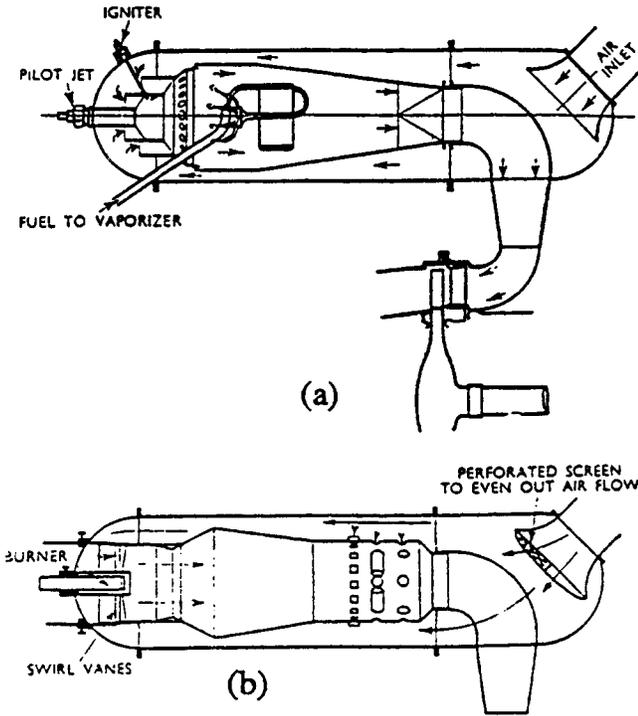
Figure 47. Vaporizer Type Combustor and Shell Type Combustor with Atomizer. (Meher-Homji, 1997; Courtesy ASME)
