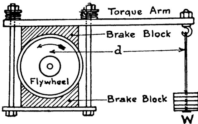
Figure 7. Prony Brake (1822) That Allowed the Scientific Testing of Turbomachines.
