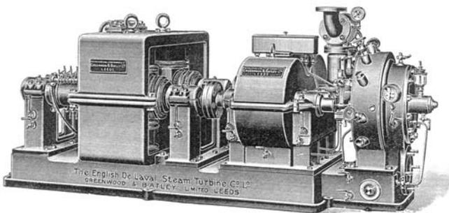
Figure 12. 150 KW De Laval Steam Turbine Turboalternator Skid. (Garrett, 1906)
