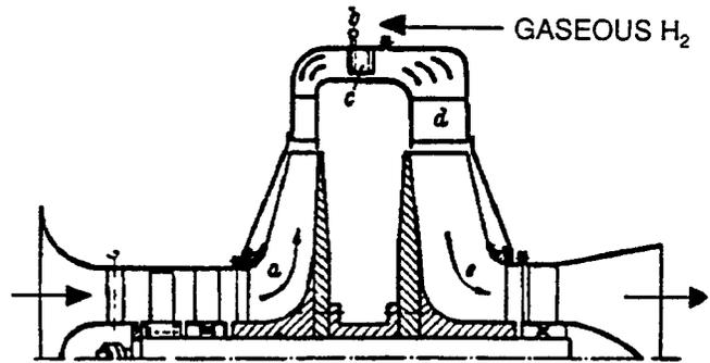
Figure 54. HeS 1 Hydrogen Fueled Demonstrator First Run in Spring 1937. (Thrust 250 lb, 10,000 rpm, and rotor diameter 12 inches.) (Meher-Homji, 1999; Courtesy ASME)
