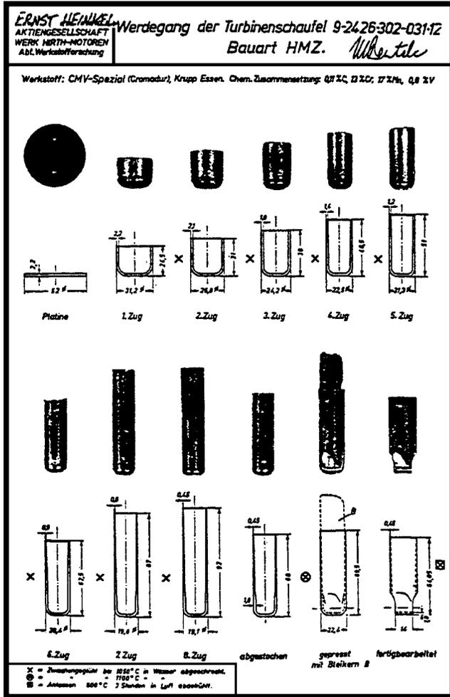
Figure 66. Ingenious Method of Developing Air-Cooled Turbine Blade Starting with a Circular Plate of 25 MM (.98 Inch) Diameter. (Hirth-Moteren Report 1944a, 1944b)
