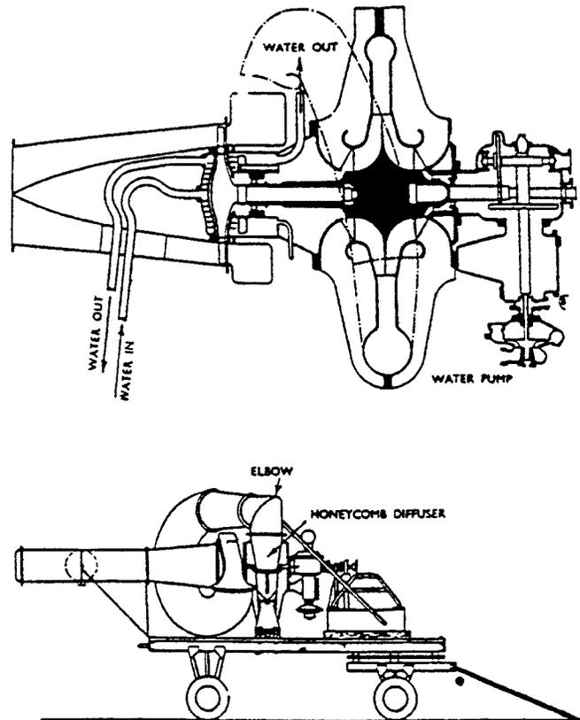
Figure 34. First Model of Experimental Engine and Test Stand, Water-Cooled Turbine Disk Jacket and Mass Flow Rate of 26 Lb/Sec. (Meher-Homji, 1997; Courtesy ASME)
