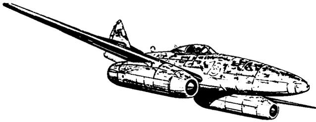
Figure 69. Messerschmitt ME-262 Fighter, the World's First Operational Jet Fighter Powered by Two Junkers Jumo 004B Turbojets. (The aircraft was capable of 550 mph and became operational in 1944.) (Meher-Homji, 1996; Courtesy ASME)
