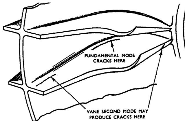
Figure 41. Position of Centrifugal Impeller Cracks. (Voysey 1945; Courtesy IMechE, UK)
