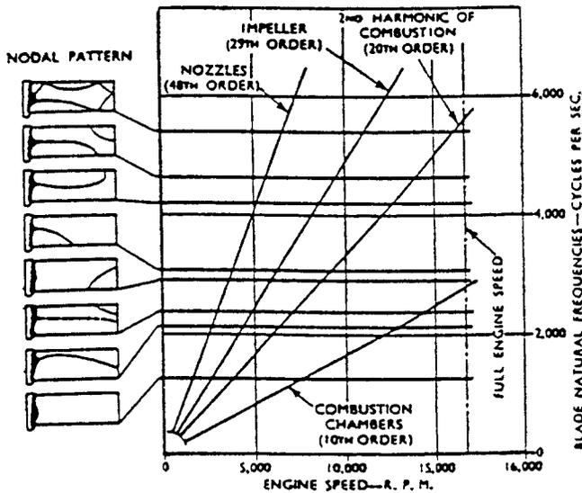
Figure 43. Interference Diagram for Turbine Blading. (Voysey, 1945; Courtesy IMechE, UK)
