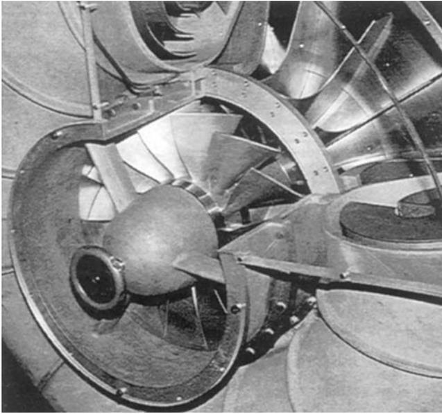
Figure 56. Inlet Section of the HeS 3B Engine Showing Axial Inducer and Centrifugal Compressor. (Meher-Homji, 1999; Courtesy ASME)
