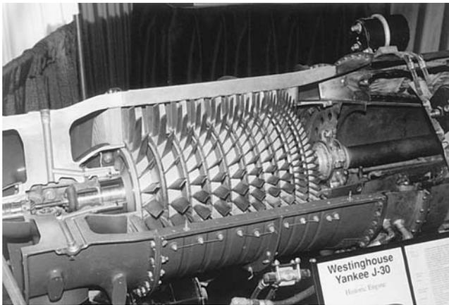
Figure 71. Westinghouse J-30 “Yankee” 10-Stage Axial Flow Compressor (Pressure Ratio of 3.8:1), Cutaway View.
