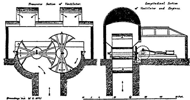
Figure 24. Early Roots Blower Used for Mine Ventilation. (Early Roots Brochure, Undated)
