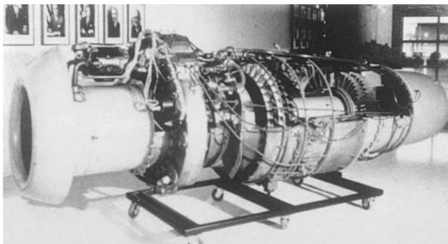
Figure 62. The Heinkel Hirth HeS 011 Engine Designed by Hans von Ohain and Max Bentele. (This was the most advanced turbojet at the end of the war, with a pressure ratio of 4.2:1, 64 lb/sec and thrust of 2863 lb.) (Meher-Homji, 1999; Courtesy ASME)
