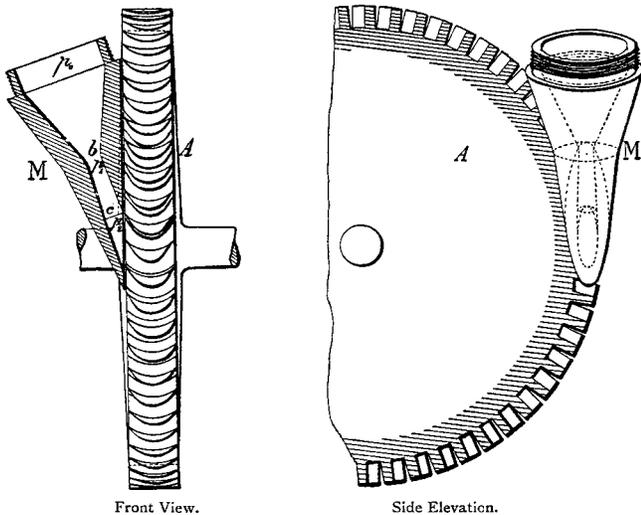
Figure 11. De Laval Impulse Turbine Wheel and Steam Expansion Nozzle. (Kennedy, 1910)
