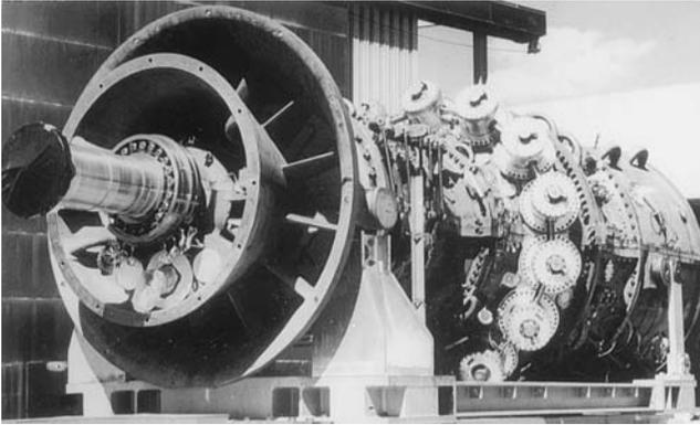
*Figure 77. Advanced GE Frame 9H Gas Turbine (Airflow Rate 1519 Lb/Sec and Pressure Ratio of 23:1), Steam Cooled Nozzles and Blades. (Courtesy GE)*
