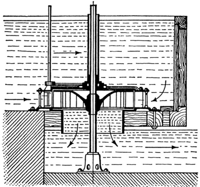
Figure 8. Francis Type Hydraulic Turbine. (Burstall, 1963)
