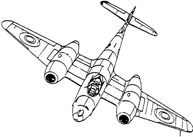
Figure 37. The First Operational Allied Fighter During WW II, the Gloster Meteor, Powered by Two Whittle W.2 Engines Built by Rolls Royce. (Maximum speed 410 mph at 10,000 ft.) (Meher-Homji, 1997; Courtesy ASME)
