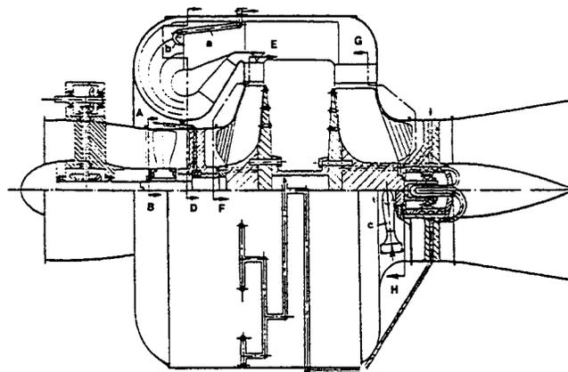
Figure 55. Layout of HeS 3B Flight Engine. (Engine speed 13,000 rpm, static thrust 1100 lb.) (Bentele, 1991)
