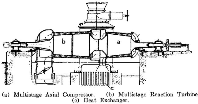
Figure 28. Stolze Gas Turbine Arrangement (Circa 1900)—10-Stage Axial Flow Compressor (Pressure Ratio 2.5:1), 15-Stage Reaction Turbine, and Silo Combustor. (Sawyer 1945)
