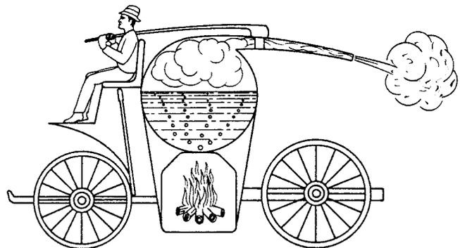
Figure 4. Newton’s Steam Carriage—Developed by Jacob Graves. Speed Control by Steam Cock.
