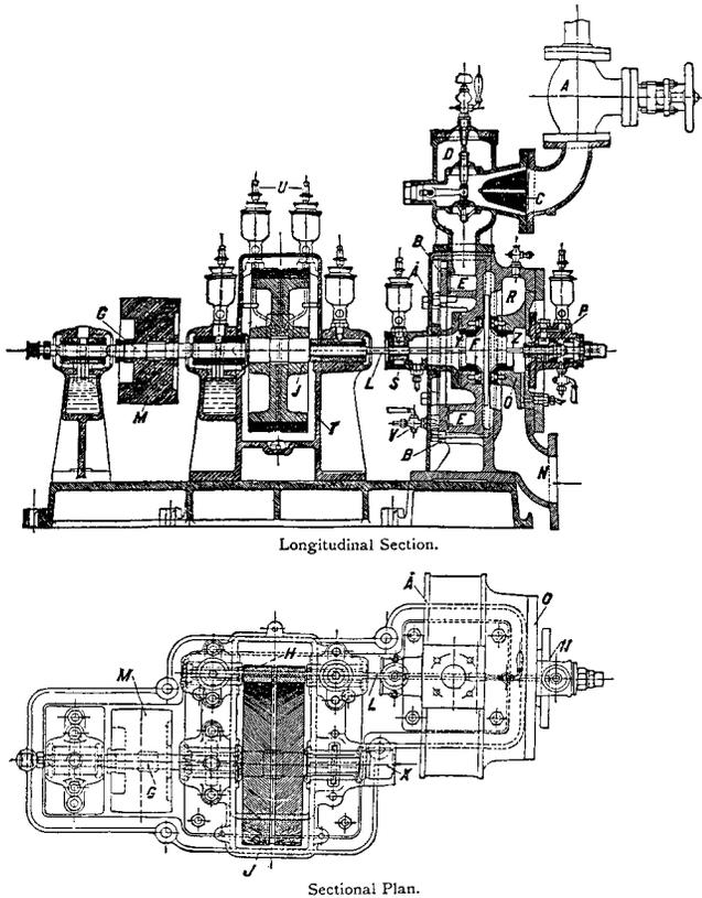
Figure 15. Longitudinal Section and Plan View of De Laval Steam Turbine Including Double Helical Reduction Gearing. (French, 1908)
