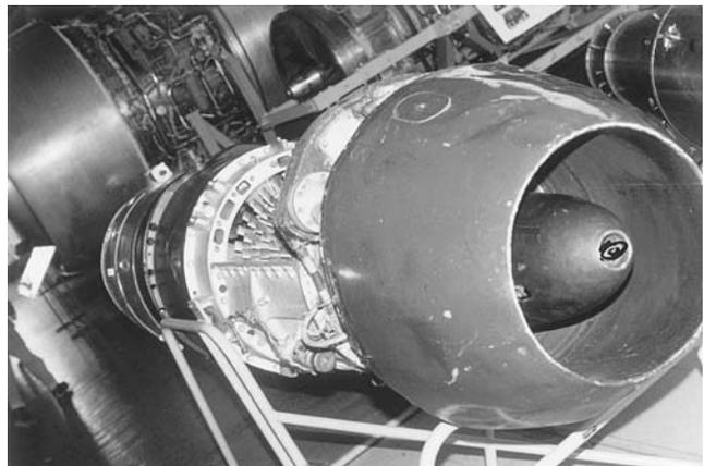
Figure 68. The Junkers Jumo 004 Engine. (1989 lb static thrust, pressure ratio of 3:1, air flow rate 46 lb/sec, 8700 rpm. Cable pull starter for the 10 hp Riedel starter motor can be seen in the nose cone.)
