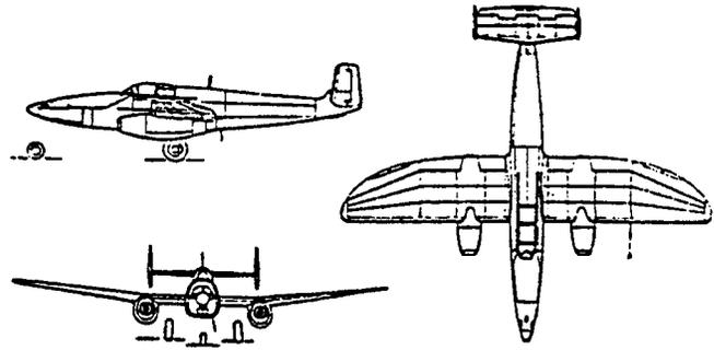
Figure 61. The Heinkel He 280 Jet Fighter Powered by Two HeS 8 Turbojets. (This fighter flew in March 1941, but production was canceled to focus on the Messerschmitt ME-262.) (Meher-Homji, 1999; Courtesy ASME)
