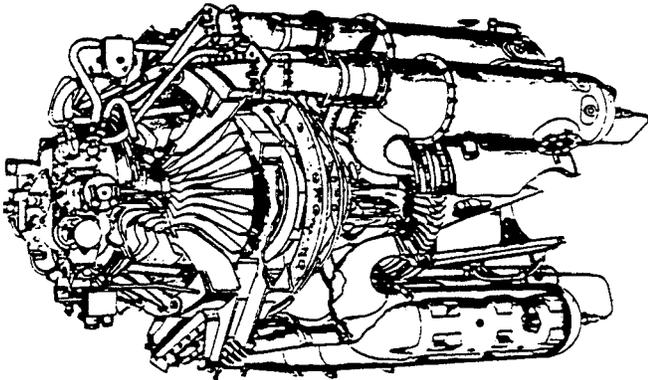
Figure 38. W.2/700 Turbojet, the Last Engine to be Built by Power Jets Limited. (Rated at 2500 lb thrust.) (Meher-Homji, 1997; Courtesy ASME)
