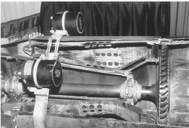
Figure 72. Westinghouse J-30 “Yankee” Annular Combustor.
