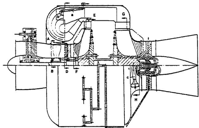
Figure 55. Layout of HeS 3B Flight Engine. (Engine speed 13,000 rpm, static thrust 1100 lb.) (Bentele, 1991)
