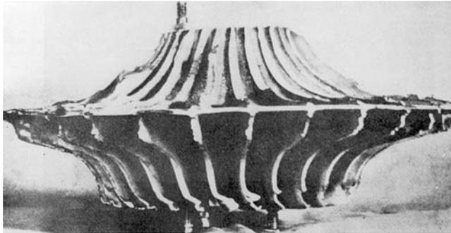
Figure 44. Impeller Failure Due to Fatigue. (Development of the British Gas Turbine Unit, 1945; Courtesy IMechE, UK)
