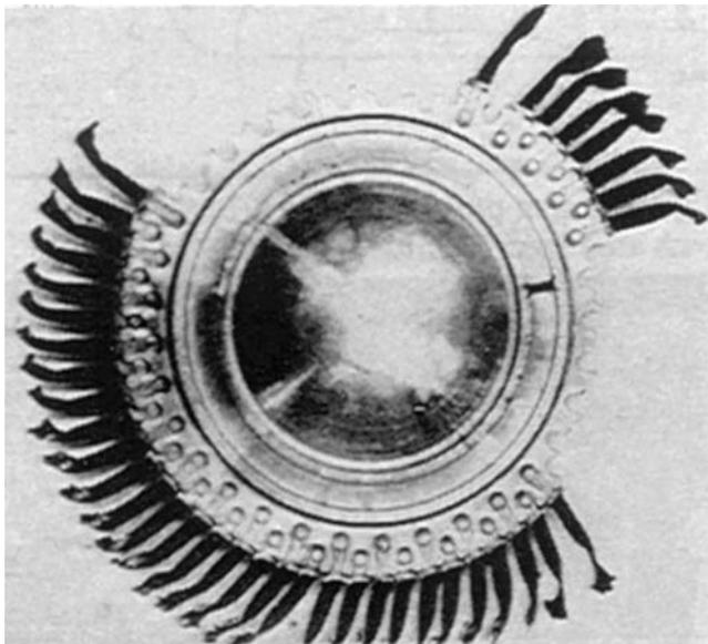
Figure 45. Disk Failure of Experimental Engine (De Laval Type Pin Blade Attachment) After 168 Run Hours. (Development of the British Gas Turbine Unit, 1945; Courtesy IMechE, UK)
