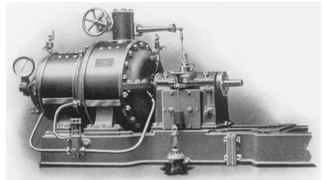
Figure 23. 60 BHP Rateau Steam Turbine. (French, 1908)
