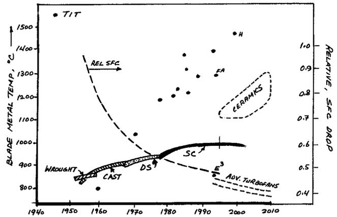
Figure 76. Turbomachinery Development for Aircraft Engines, 1940 to Present, Including SFC, TIT, and Material Capability.
