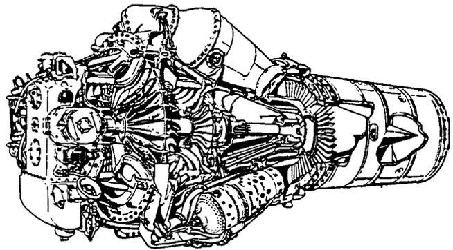
Figure 39. Cutaway of the Rolls Royce Nene Engine (5000 Lb Thrust, 80 Lb/Sec), Designed by Sir Stanley Hooker Incorporating Basic Whittle Design Features. (Meher-Homji, 1997; Courtesy ASME)
