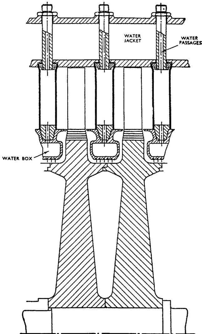
Figure 52. Details of Experimental British Water-Cooled Gas Turbine Developed in the Early 1940s. (Constant, 1945; Courtesy IMechE, UK)
