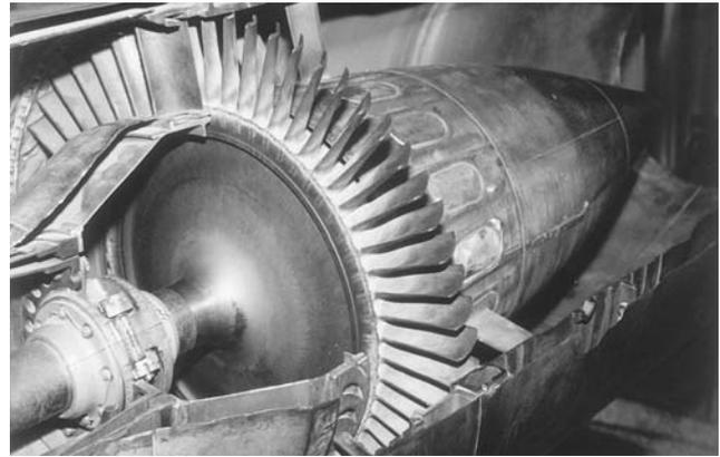
Figure 73. Westinghouse J-30 “Yankee” Single-Stage Turbine Wheel (17,000 RPM) and Jet Pipe.
