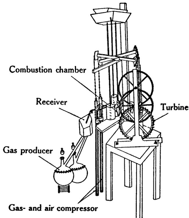
Figure 5. Patent Drawing of John Barber (1791) of Gas Turbine Cycle Utilizing Reciprocating Compressor, Combustor, and Turbine.
