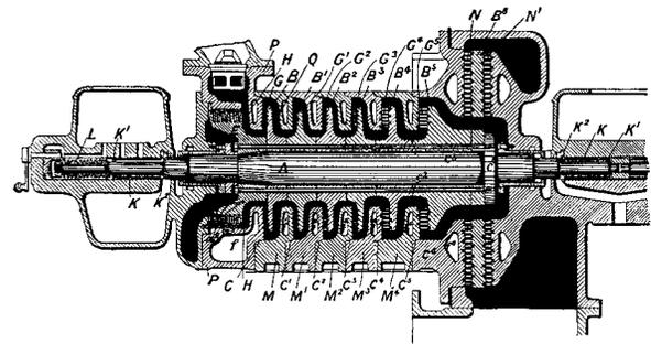
Figure 17. Parsons' Radial Flow Compound Turbine. (Kennedy, 1910)
