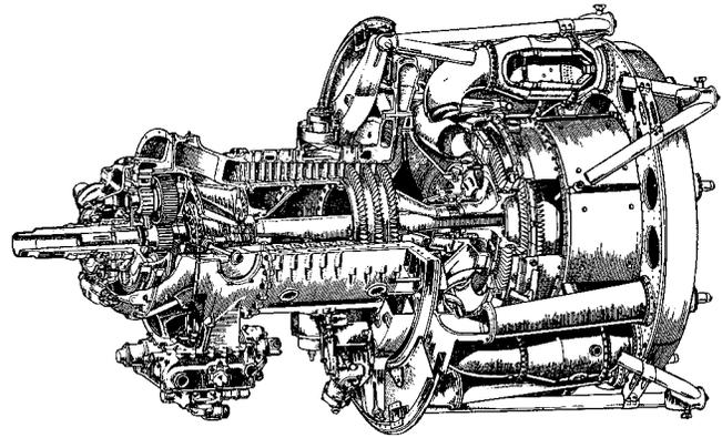
Figure 49. Sectioned View of the Bristol Theseus Axial Flow Turboprop Engine. (Geoffrey Smith, 1946)
