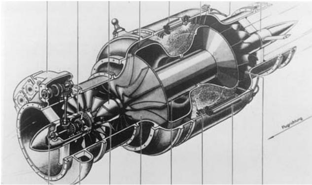
Figure 60. HeS 8 Turbojet Designed by von Ohain (13,500 RPM), Designed to Power the World's First Jet Fighter, the He 280. (Meher-Homji, 1999; Courtesy ASME)
