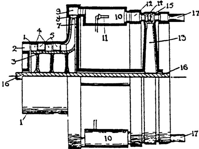
Figure 33. Whittle Patent Drawing (1930) Showing Two-Stage Axial Compressor, Centrifugal Compressor, Straight-Through Burner, and Two-Stage Axial Turbine on One Disk. (Meher-Homji, 1997; Courtesy ASME)
