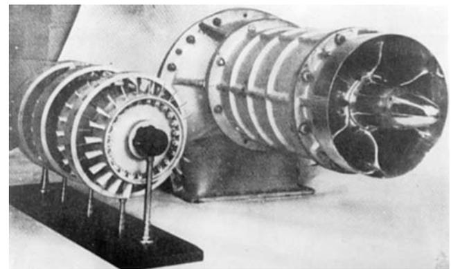
Figure 51. Six Inch Diameter Experimental Multistage Axial Flow Compressor, "Anne," First Run in 1938. (Tip speed 750 fps, 28,600 rpm.) (Constant, 1945; Courtesy IMechE, UK)
