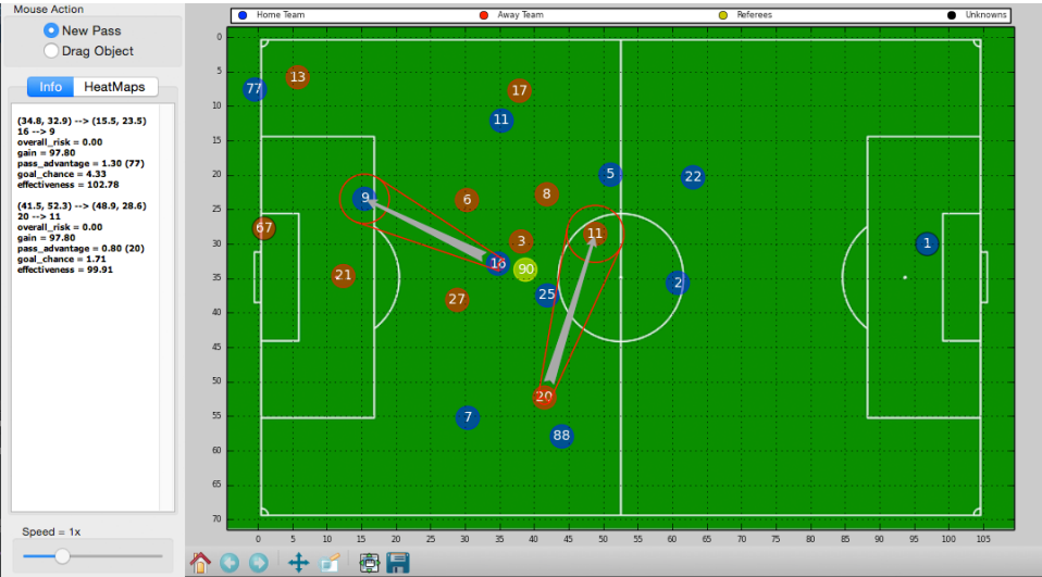
Fig. 5. (Color online) Pass risk area visualization for manually defined passes — For each pass, the red lines indicate the borders of the risk area in which an opponent player may pose a threat to the pass.
