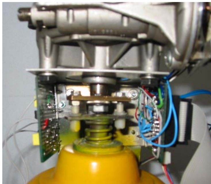
Picture 2.12: The coupling between gear and handle bar
