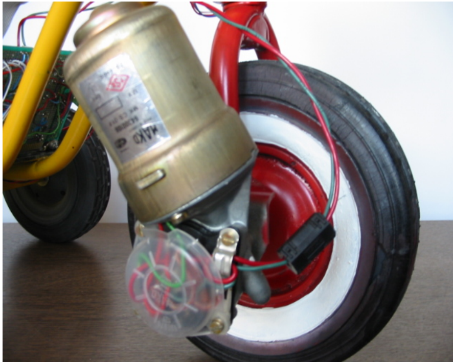
Picture 2.2: The motor pedestal providing the movement of the front wheel
