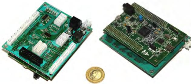
Fig. 3: Custom flight control computer (FCC) hardware
