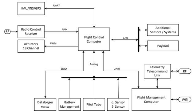
Fig. 4: Hardware architecture of Flight Management System
