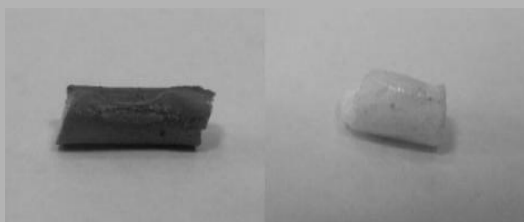
Photographs of the freeze-dried hydrogels with (Gel-9) or without (Gel-10) Ag NPs.
