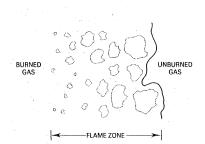
Turbulent flame speed is in the range of 50 - 60 m/s
