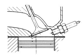
**Wedge Shaped Combustion Chamber**
