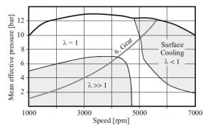
Modes of operation in the characteristic map of a DISI engine acc. to Fröhlich et al. (2003)
