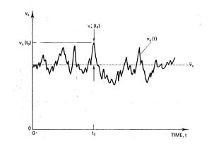
$$\overline{\phi} \equiv \frac{1}{\Delta t} \int_{t_1}^{t_2} \phi(t) dt$$
