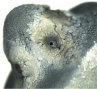
Fig. 3.1b. Deposits at a diesel injector tip. (Copyright by Afton Chemical Ltd. Reproduced with permission.)
