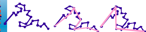
Figure 8.2 Line generalization alternatives. The line (left) can be resampled by retaining every n th point (center), or by repeatedly selecting the most distant point from a line between end nodes (right) and redividing the line until a minimum distance is reached, the Douglas-Peucker method.
