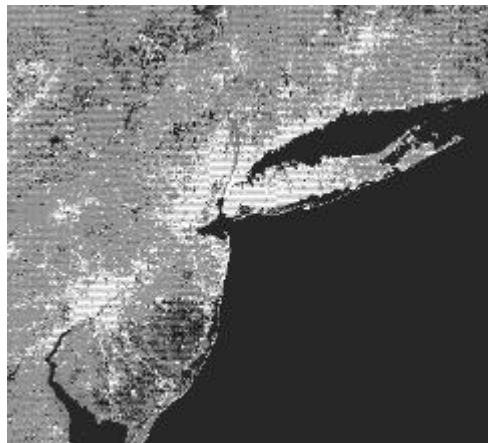
Figure 3.8 GIS data layer as a grid with a large section of “missing data,” in this case, the zeros in the ocean off of New York and New Jersey.
