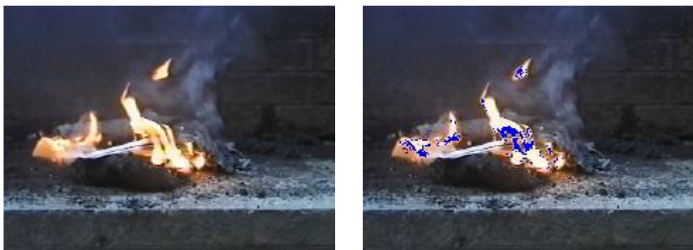
Figure 16. Detection of Fire Pixels, Example 1
