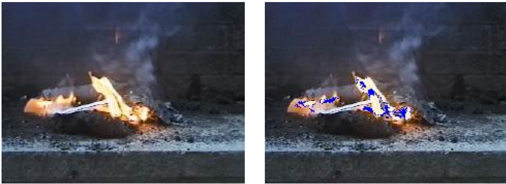
Figure 16. Detection of Fire Pixels, Example 1
