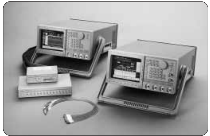
▶ Figure 42. Pattern generators and external signal interface "pod".
