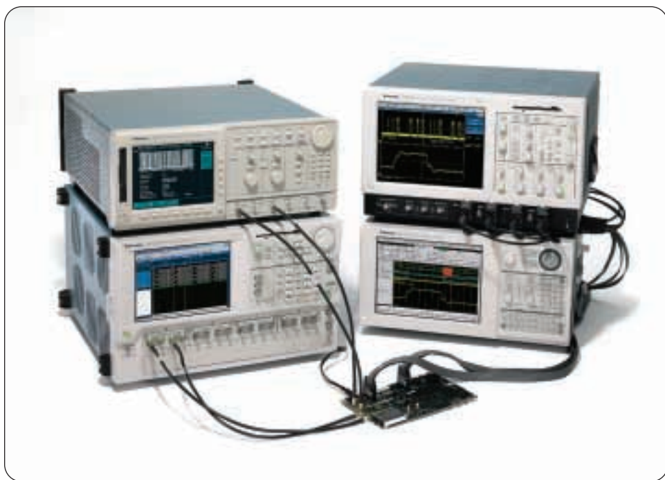
▶ Figure 1. Most measurements require a solution made up of a signal source paired with an acquisition instrument. Triggering connectivity simplifies capturing of the DUT output signal.
