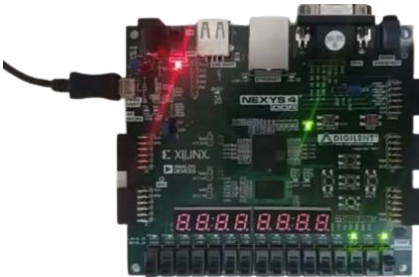
Figure 4.7 : 0x5 value on the LEDs.
