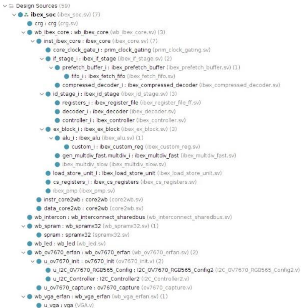
Figure 4.13 : Vivado Wishbone project hierarchy.
