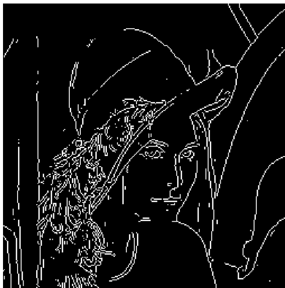
Figure 3.11 : Gradient magnitude of the cover image from Sobel operator.
