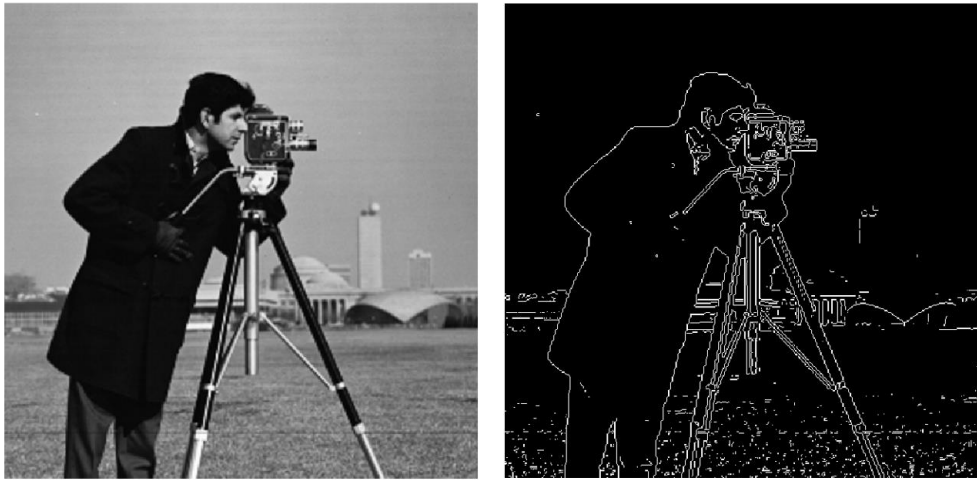
Figure 3.5 : Grayscale image and its gradient magnitude from Sobel operator [15].
