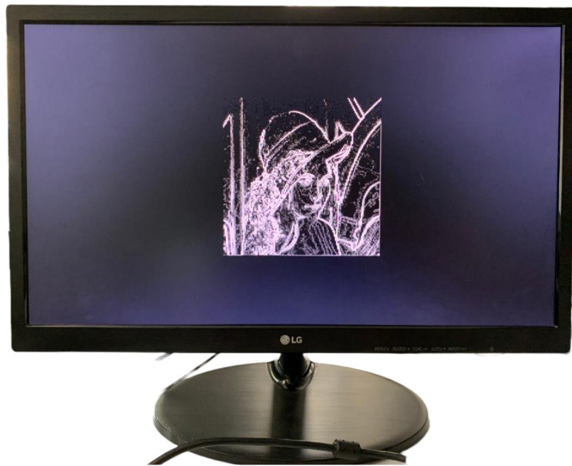
Figure 5.26 : Sobel filter output given to the monitor.
