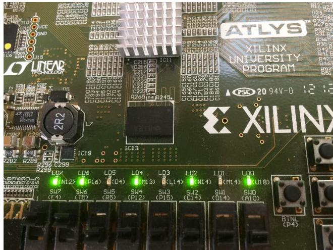
**Figure 2.18 :** Output of the Led Test application
