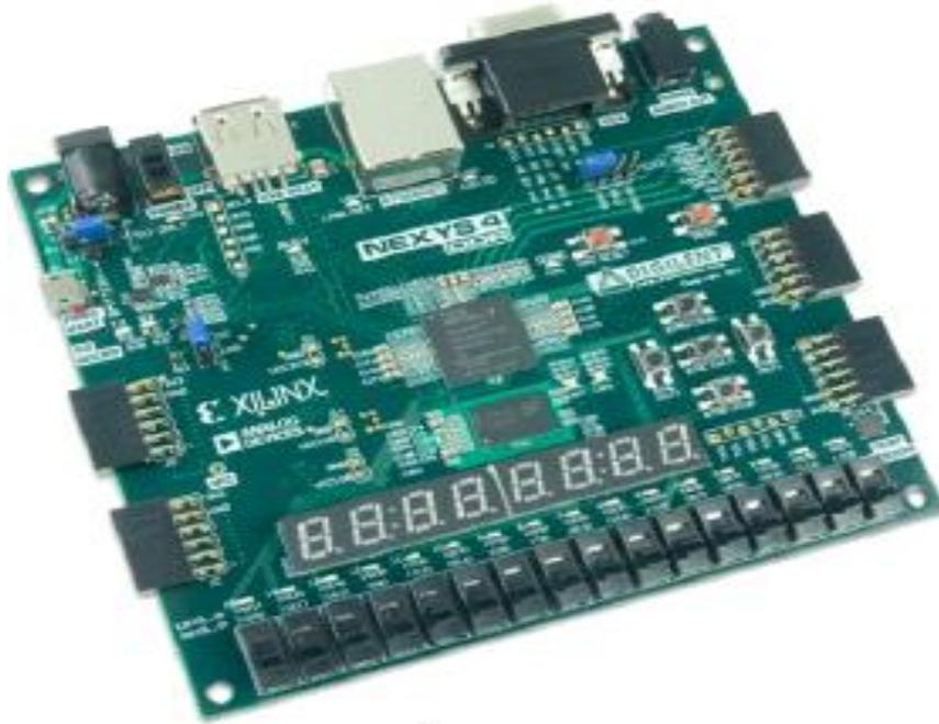
**Figure 4.1** : Nexys 4 Artix-7 FPGA Board [37]
