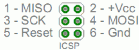
Figure 4.3: Arduino ICSP Pins [36]
