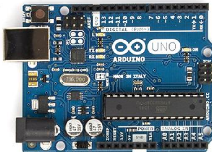
Figure 2.7: Arduino Uno R3 board [13].
