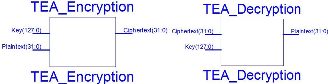
Figure 16 TEA Encryption and Decryption module RTL schematics
