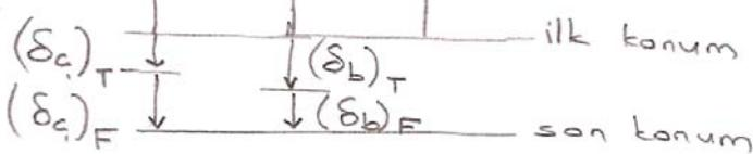
$$(\alpha \Delta T \cdot L)_q + \left( \frac{FL}{AE} \right)_q = (\alpha \Delta T L)_b + \left( \frac{FL}{AE} \right)_b$$
