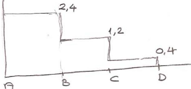
$$(b) (\bar{\tau}_{AB})_{\text{maks}} = \frac{T_{AB}}{J_{AB}} c_{AB} = \frac{2400 \times 10^3}{\frac{\pi}{2} 27^4} \cdot 27 \\ = 77,6 \text{ MPa}$$
